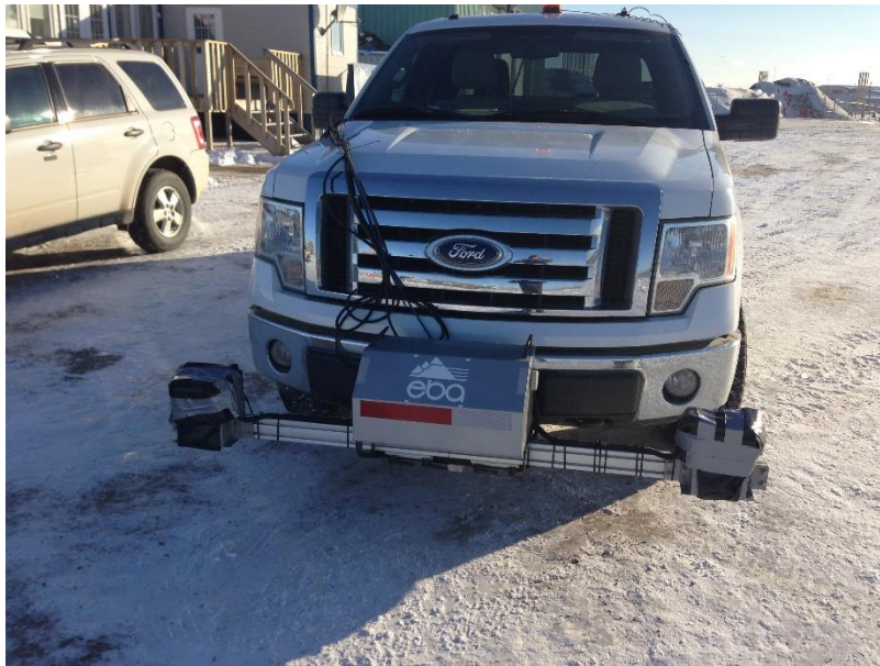
Figure 6- PSP-2000 Dual Wheel Path Inertial Profiler Integrated onto a Standard Service Vehicle
