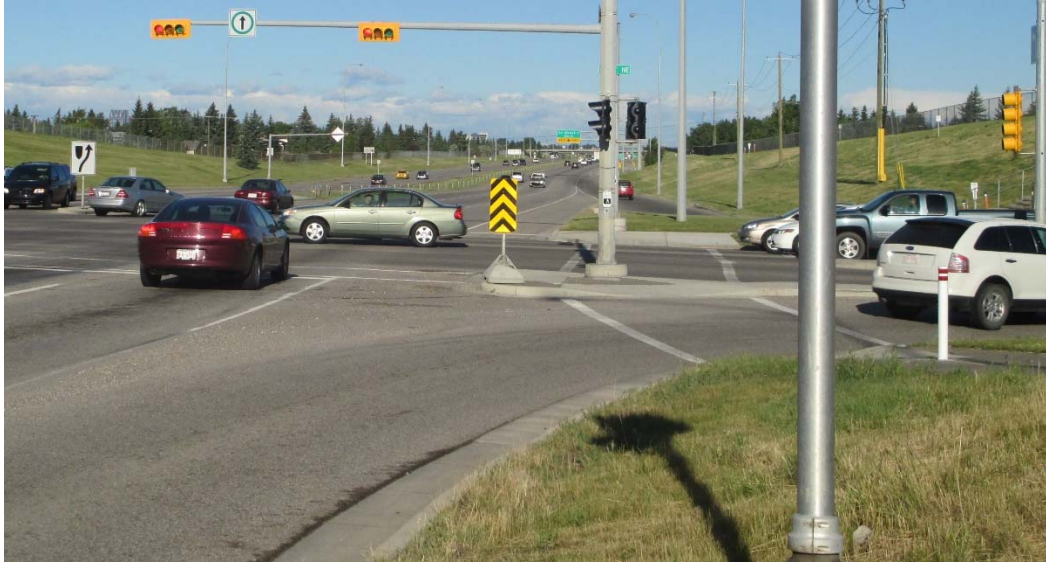
Figure 2: Small Radius Right Turn Island, with Added Lane
