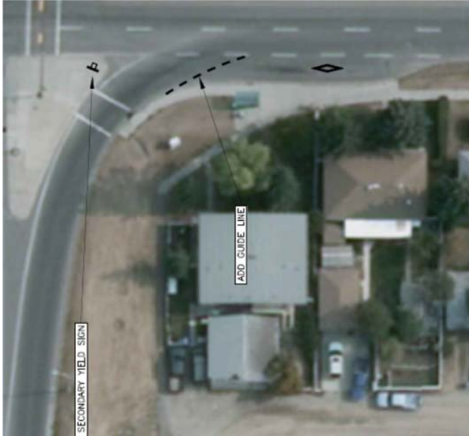
Figure 5: Mitigation Option (for Figure 4 scenario) - Guide Lines and Bus Bay Diamond
