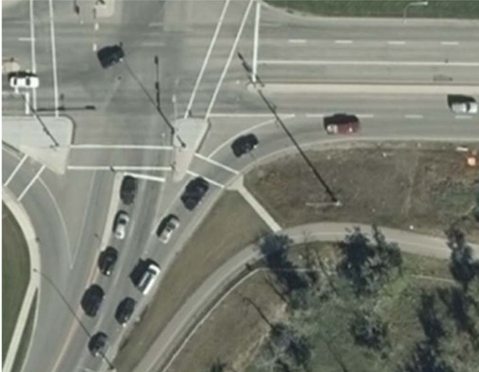
Figure 3: No Deflection on Right Turn Island (centre of photo), with Added Lane
