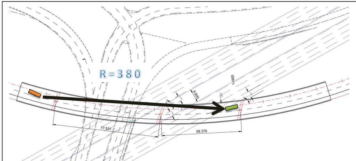
Figure 7: Inadequate stopping sight distance due to visual interference from F-shape barriers.
