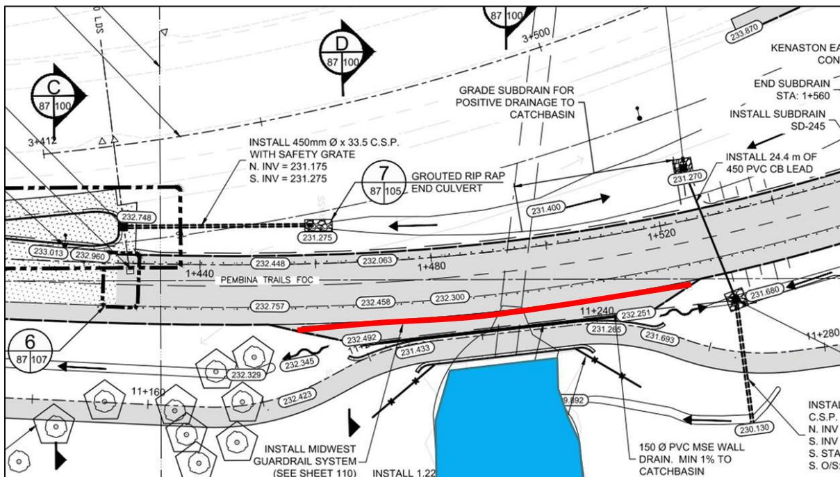
Figure 11: AT path must come in tight over the box culvert. Note “Midwest Guardrail System” highlighted in red for protection from vertical drop.
