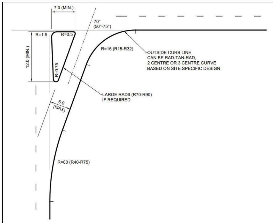
*Figure 3: Typical Smart Channel Geometry (Source: City of Winnipeg “(Draft) Transportation Standards Manual – 2012 Update”. Drawing No. SI-14).*
