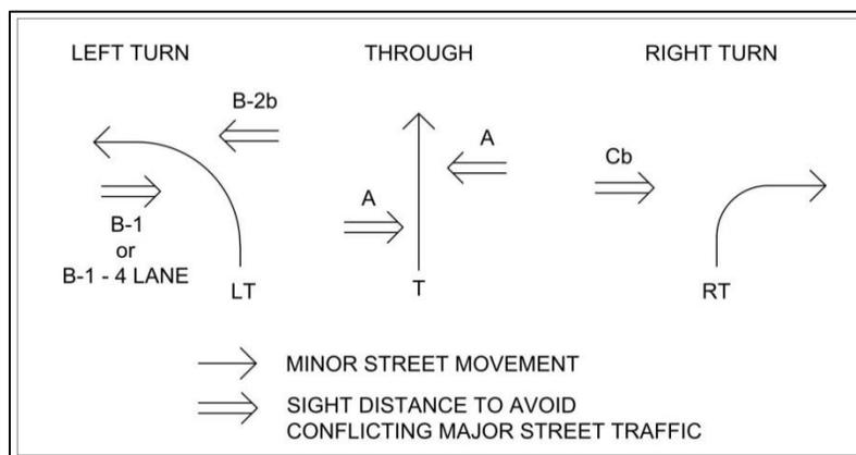
Figure 2: Sight Distance Parameters for Turning Movements from Stop Condition.
