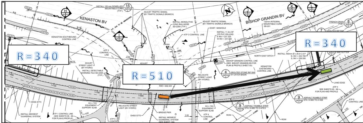
*Figure 8: Adequate stopping sight distance achieved through combination of geometric changes.*
