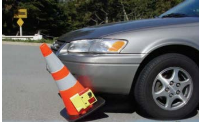
FIGURE 3 Work zone intrusion alarm (7).
