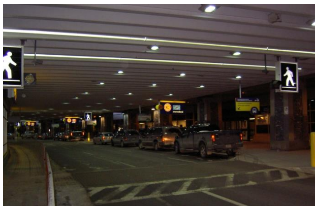
Photo 19: Calgary – Perpetual Night Appearance, Large Columns Obstructing Views, and Low Clearance
