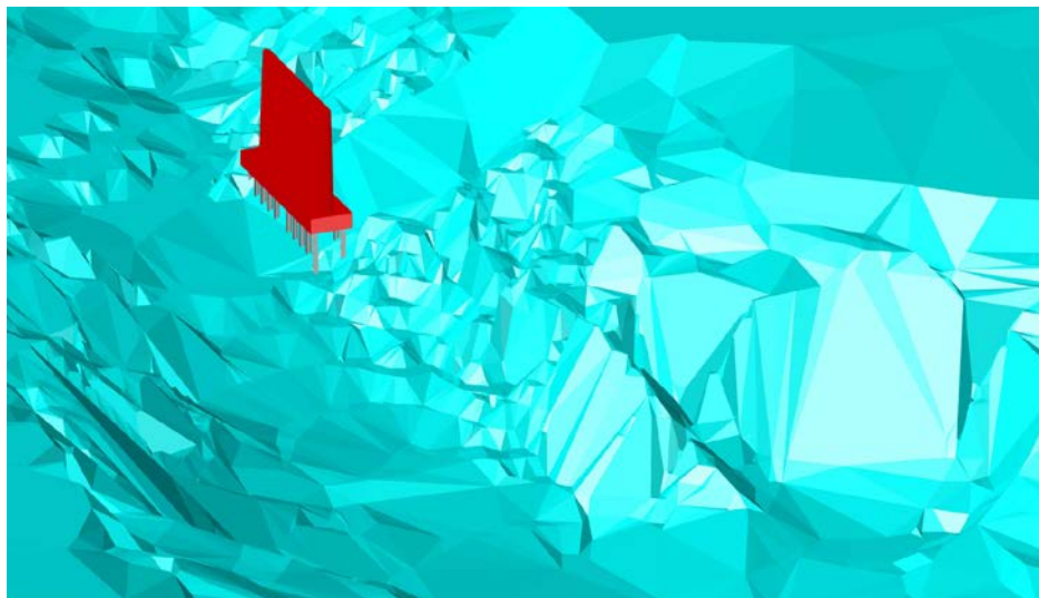
Figure 19 – Three Dimensional Image of Assiniboine River, Showing Existing SU.4 and Extent of Scouring Around Pier and Downstream of Bridge
