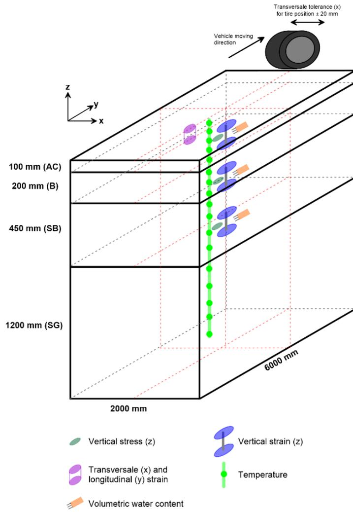
**Figure 3. Tested pavement structure**
