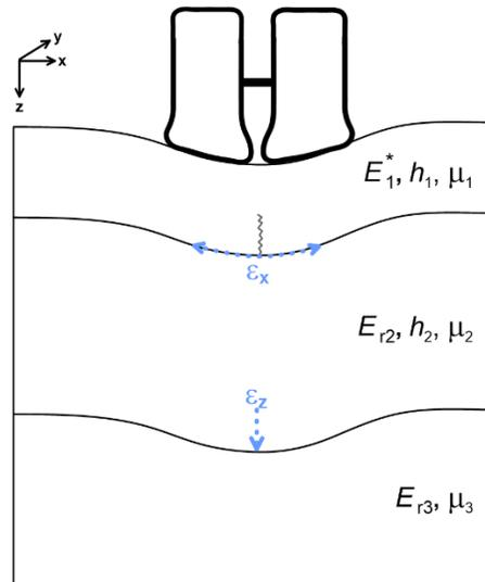
Figure 1. Tensile strain at the bottom of asphalt concrete and vertical strain at the top of the subgrade
