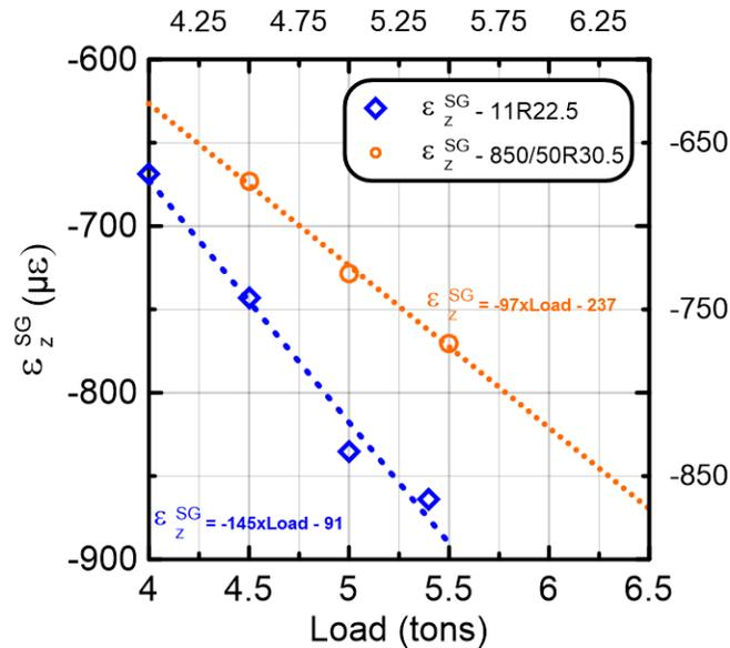
Figure 13. Example of linear trends used to obtain LLF
