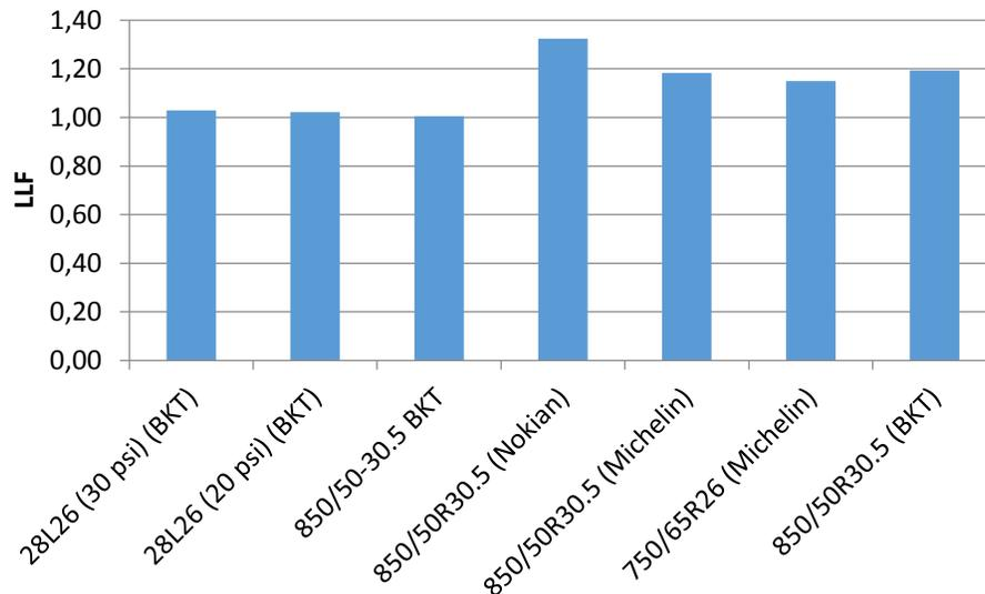
Figure 14. Load limit factor determined for a reference half-axle load of 5000 kg
