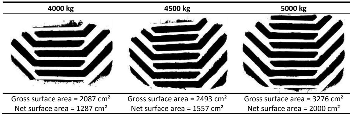
Figure 8. Example of loaded tire print measurements (850/50-30.5)
