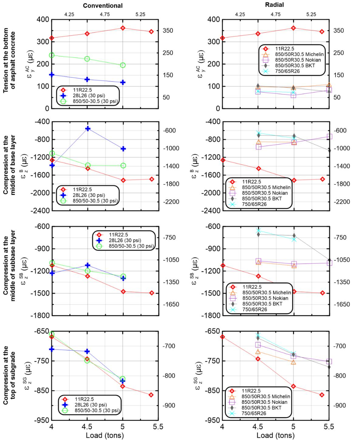
Figure 10. Strain data as a function of half-axle load for conventional and radial tires
