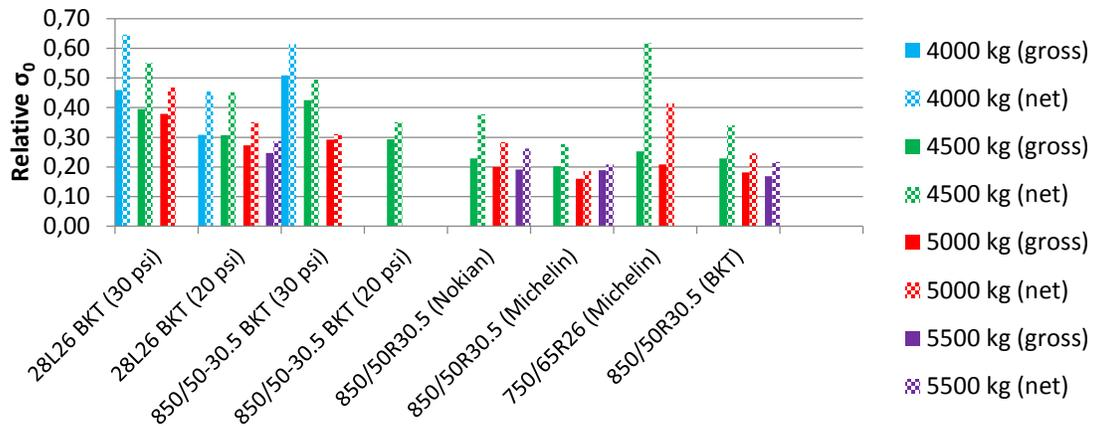
Figure 9. Relative values of surface contact stress for each tire and load considered
