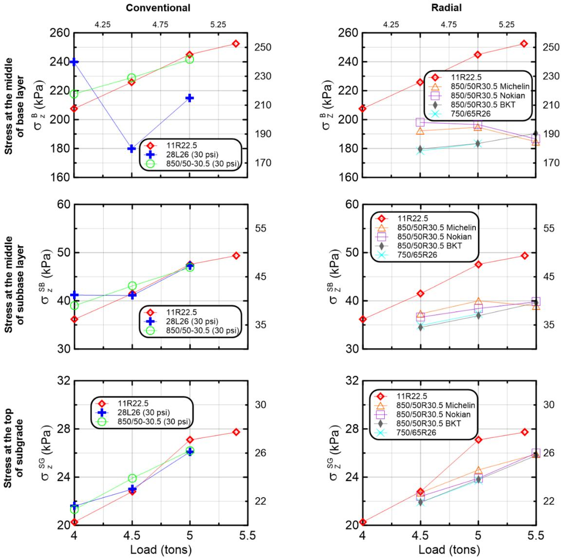
Figure 11. Stress data as a function of half-axle load for conventional and radial tires
