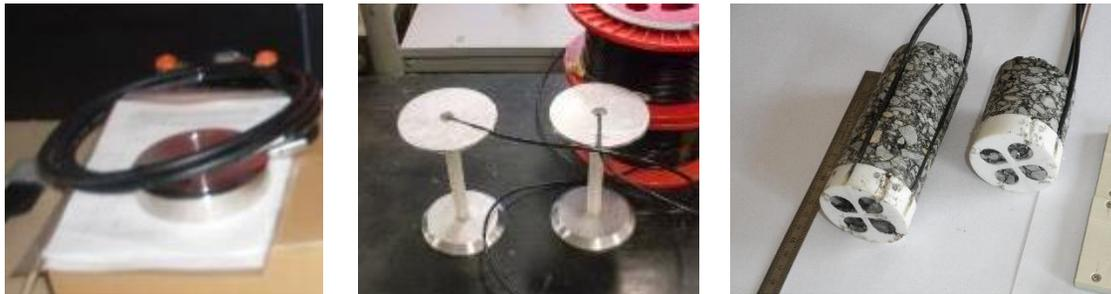
Figure 5. Mechanical response sensors – Left : Vertical stress  $\sigma_z$  in soil and unbound layers; Center : Vertical strain  $\epsilon_z$  in soil and unbound layers; Right : Transversal  $\epsilon_x$  and longitudinal  $\epsilon_y$  strain at the bottom of asphalt concrete
