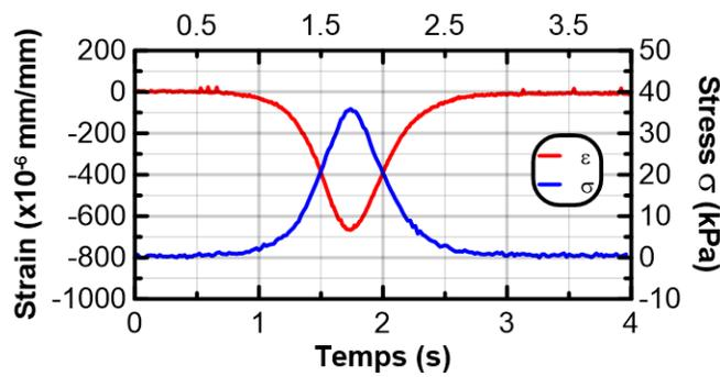
Figure 6. Example of vertical stress and vertical strain signal - Subbase
