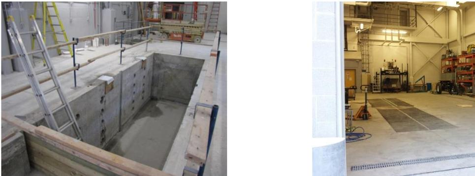
**Figure 2. Indoor test facility – Left : empty test pit; Right : Paved flexible pavement structure**
