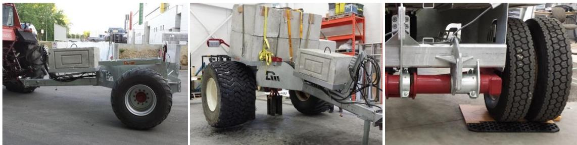
**Figure 7. Left - Farm trailer used; Center – Loading with concrete blocks; Right – Half-axle weight measurement**
