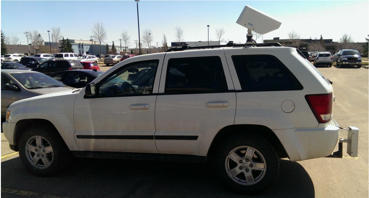
Figure 1: Vaisala DSP310 sensor mounted on small truck
