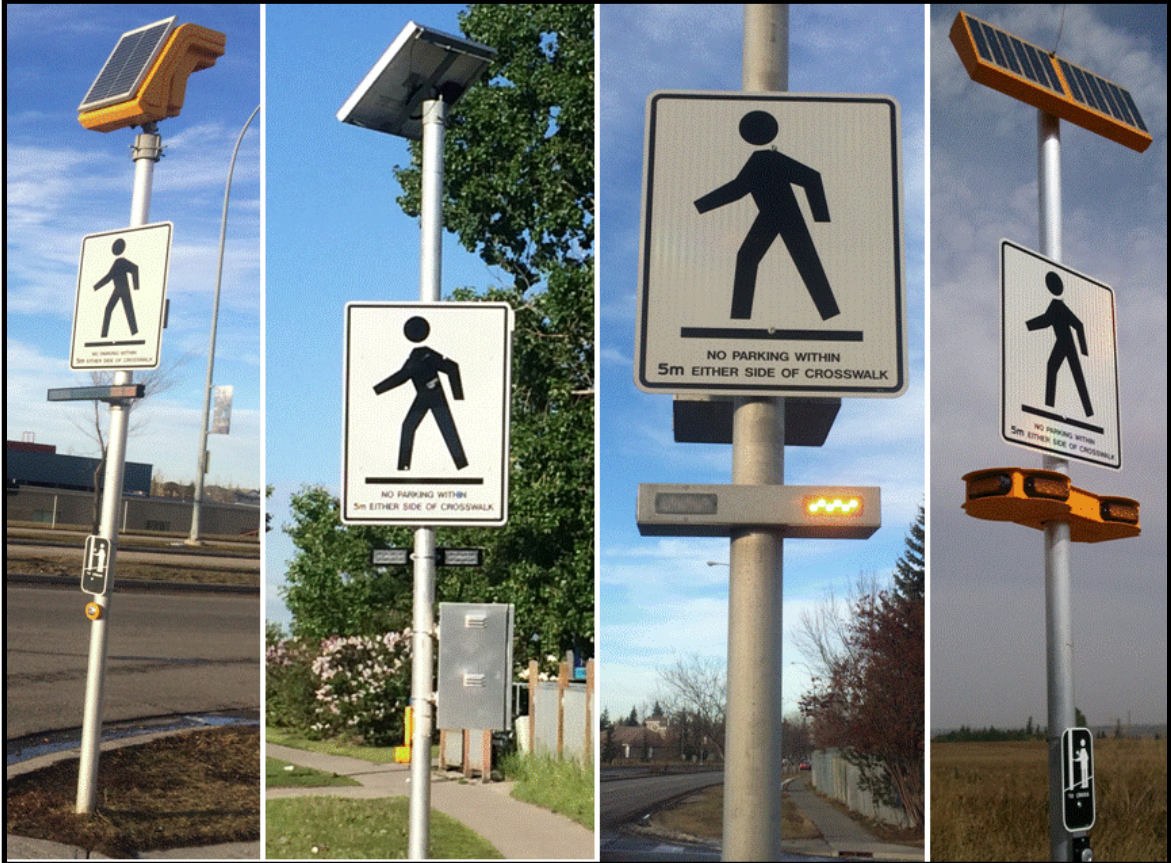
Figure 4: Various types of RRFB devices used in Calgary
