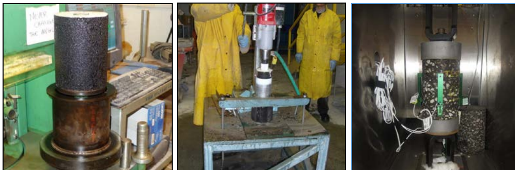
Figure 2. Dynamic modulus test samples production
