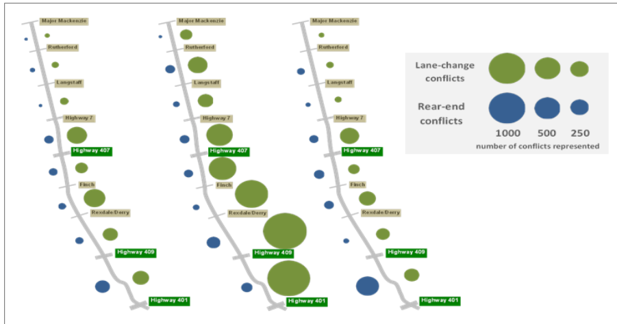
Figure 4: A plot of safety-related conflicts (produced by micro-simulation in conjunction with SSAM, the Surrogate Safety Assessment Model) for evaluation of safety related to future conditions
