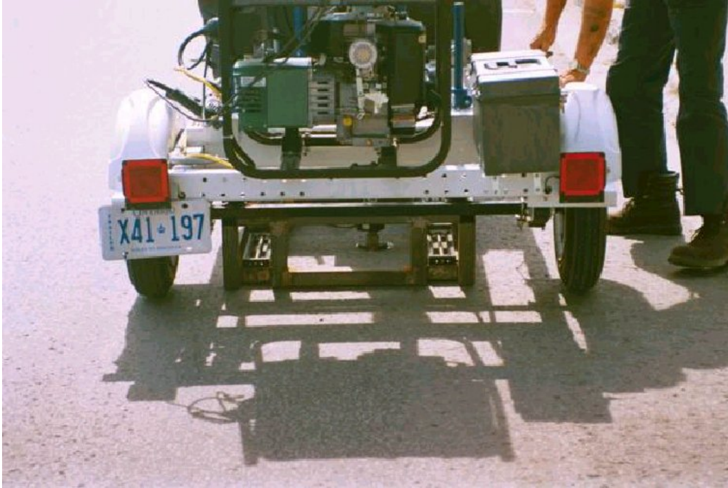
Figure 2: Applying torque to the pavement surface
