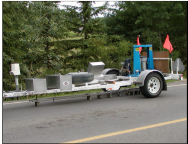
Figure - 16 Falling Weight Deflectometer Deflection Testing Apparatus
