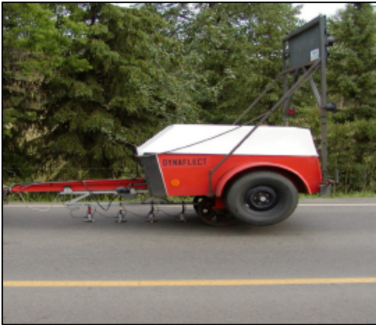
Figure 15 - Dynaflect Deflection Testing Apparatus
