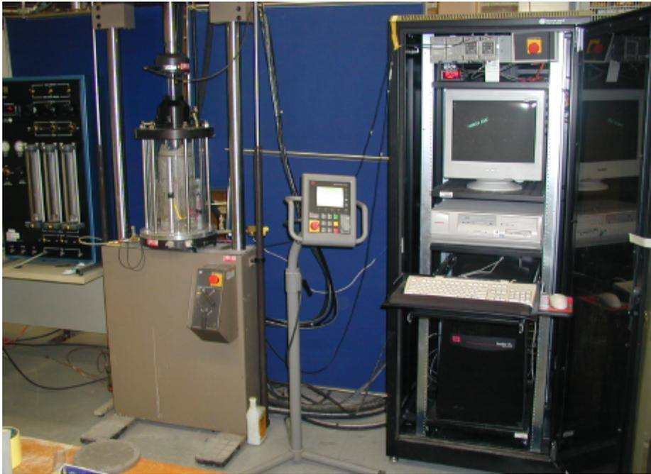
Figure 1: IRC resilient modulus test system
