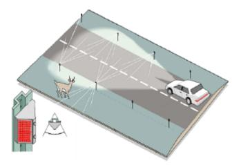
Figure 4. Light reflection concept of wildlife warning reflectors (Source: Brian Shellito, The Detroit News (copyright) (adapted) (used with permission))
