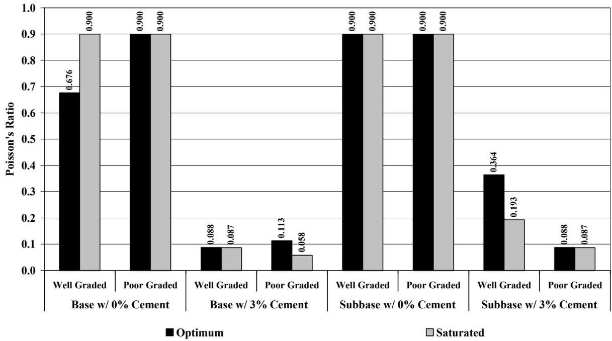
Figure 9 Mean Poisson's Ratio across Stress State and Frequency
