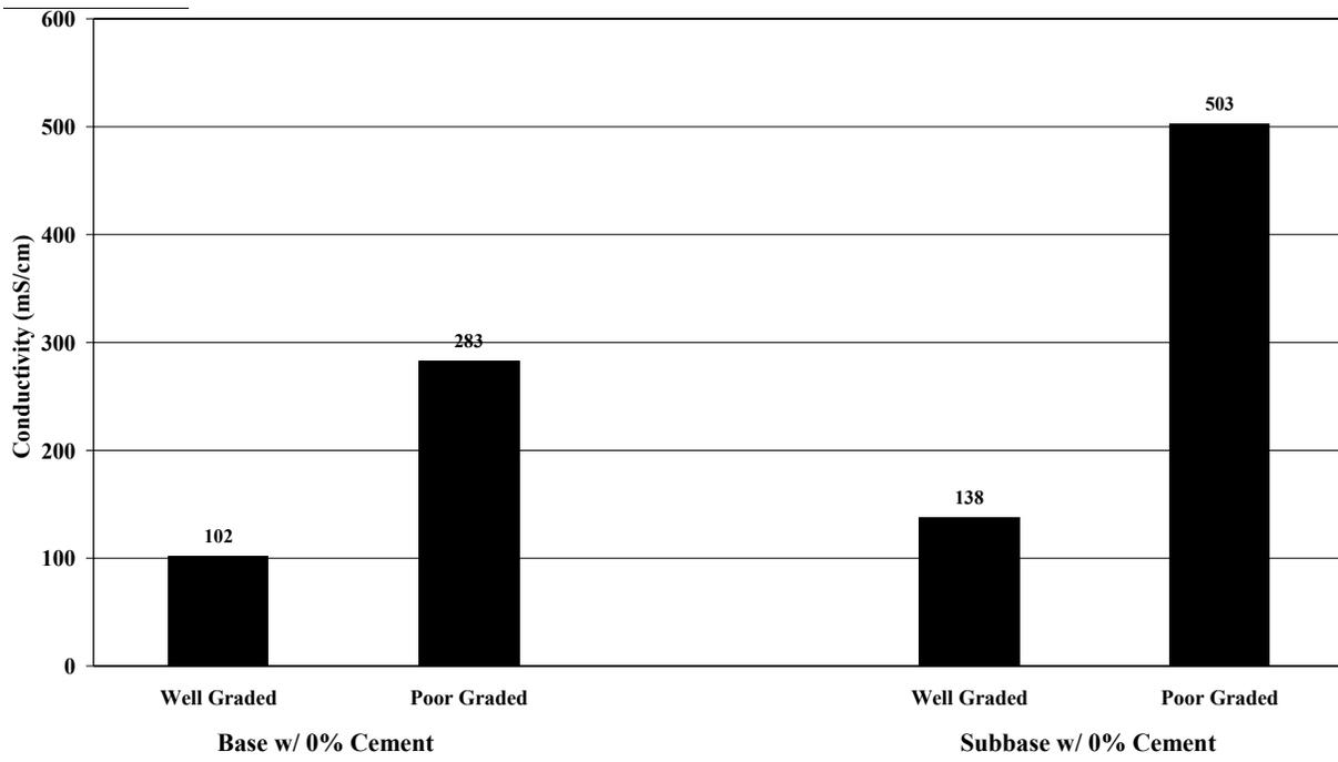
**Figure 3 Plateau Conductivity of Saturated Granular Materials**
