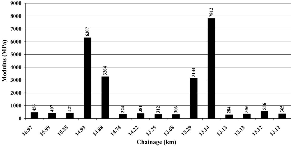
**Figure 2 Granular Base Moduli Profile of Control Section 11-06**
