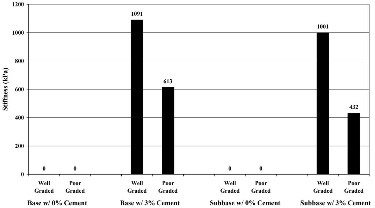
**Figure 4 Unconfined Compressive Stiffness**
