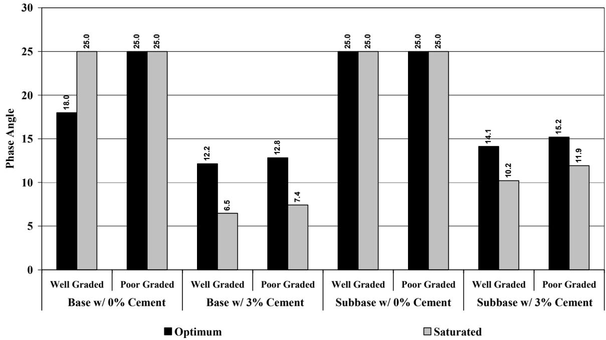
**Figure 10 Mean Phase Angle across Stress State and Frequency**
