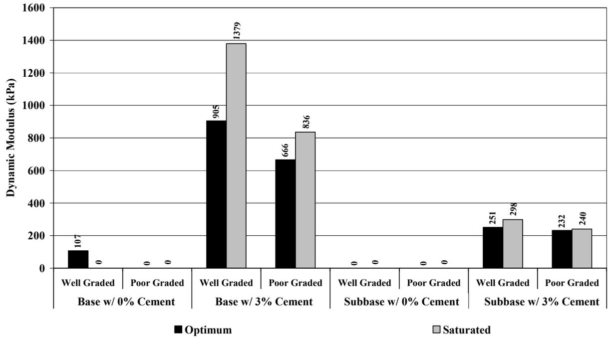
**Figure 8** Mean Dynamic Modulus across Stress State and Frequency
