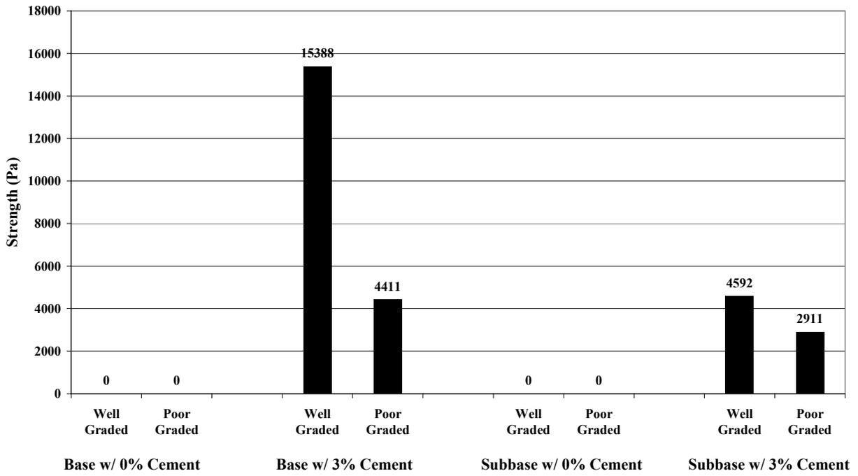
**Figure 5 Unconfined Compressive Strength**
