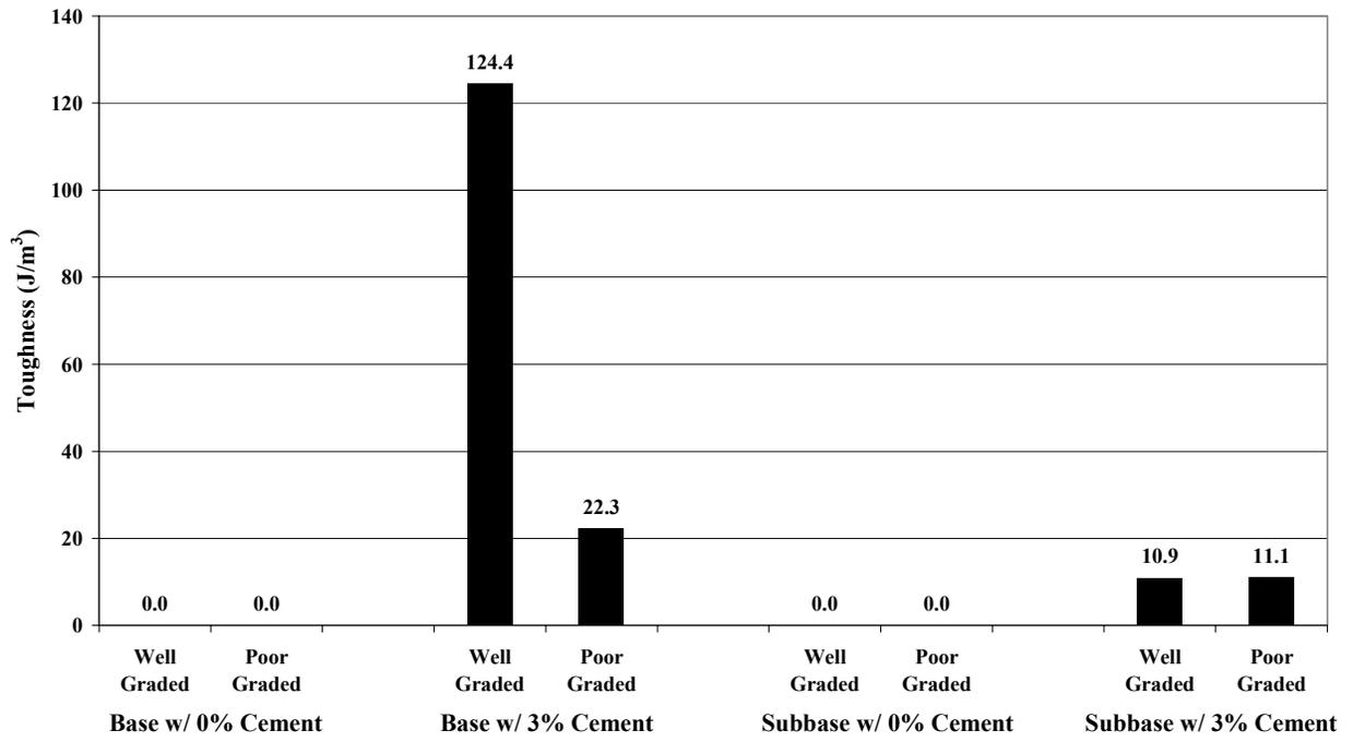
**Figure 6 Unconfined Compressive Toughness at Ultimate Strength**
