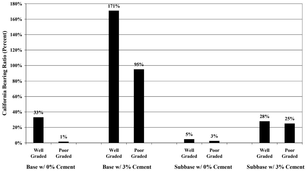
**Figure 7 California Bearing Ratio**
