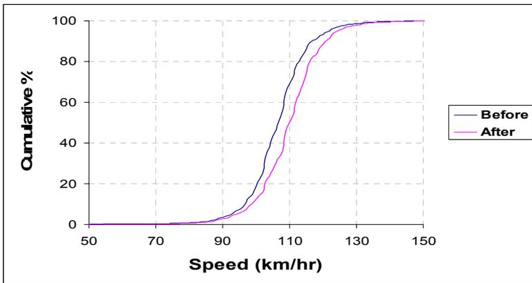
The net changes in percentile speeds from the before and after studies at the permanent traffic stations is shown in Figure 5. Individual speed records from all permanent traffic stations were combined to determine this net change. The permanent traffic stations collected extremely large speed samples resulting in large samples in each percentile speed.
