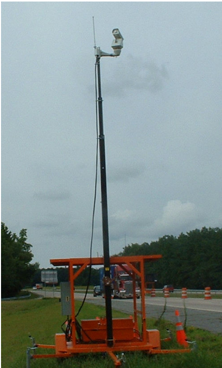
Figure 3. Portable camera trailer deployed on Interstate 95
