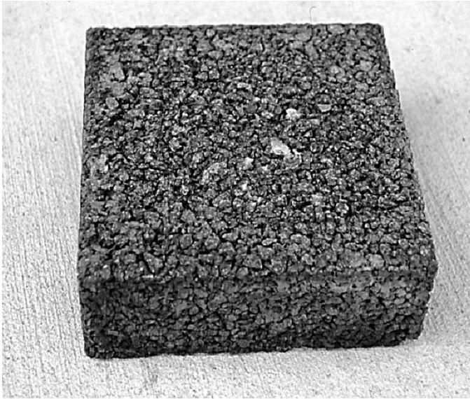
Figure VII: Porous concrete paver – these pavers are not recommended for extreme freeze/thaw climate conditions (Source: ICPI, 2000)
