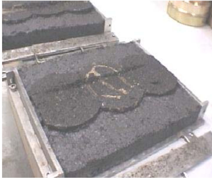
PHOTOGRAPH 4 Asphalt cylindrical samples after application of 20,000 wheel passes. (HWRT)
