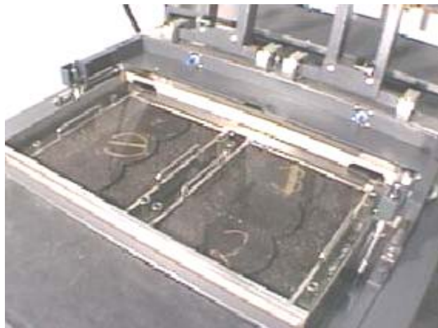
PHOTOGRAPH 3 Asphalt samples submerged in water prepared for the HWRT wet test.
