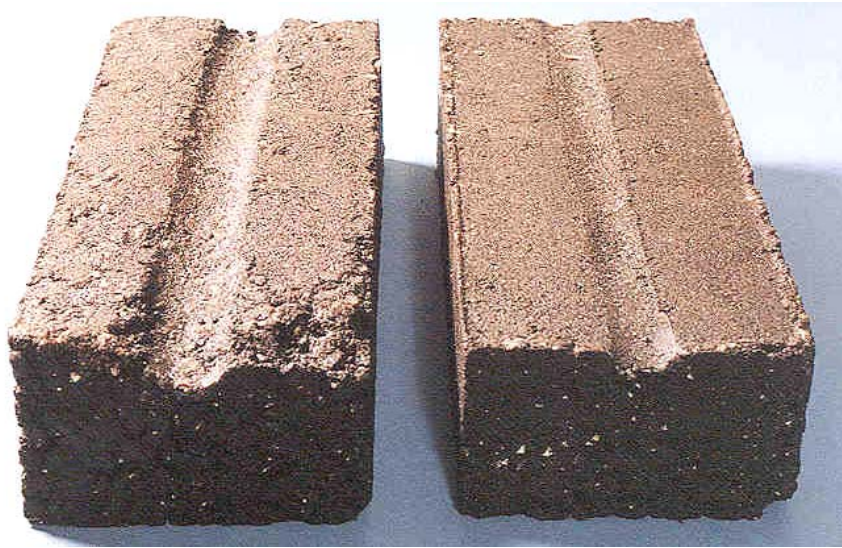
PHOTOGRAPH 9 Laboratory prepared beam samples tested in the APA. The sample on the right hand side has a better resistance to permanent deformation (rutting) than the one on the left hand side.
