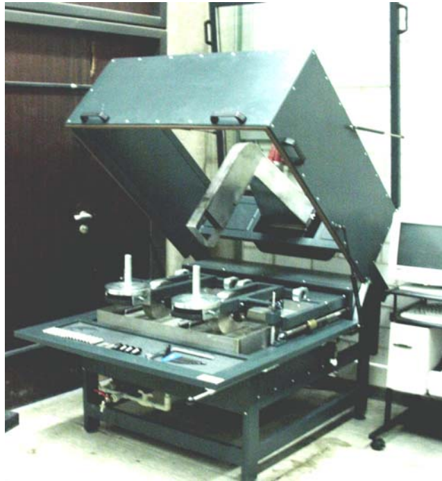
PHOTOGRAPH 2 Hamburg Wheel Rut Tester in operation.
