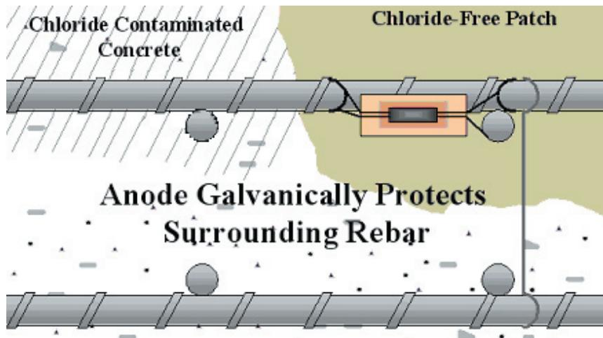
Figure 4: Installed Embedded Galvanic Anode in Patch Repair
