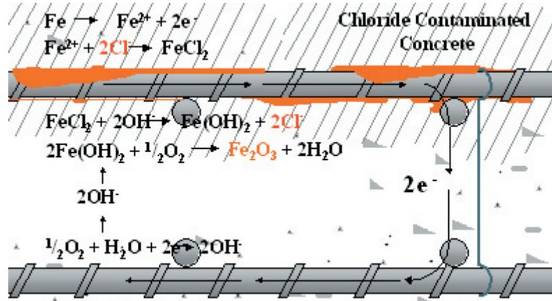
Figure 1: Typical Corrosion Cell in a Concrete Deck
