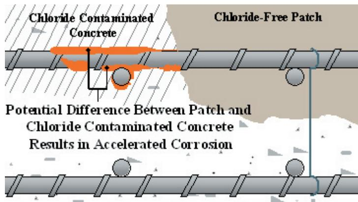
Figure 2: Ring Anode Corrosion Adjacent to Repair Patch
