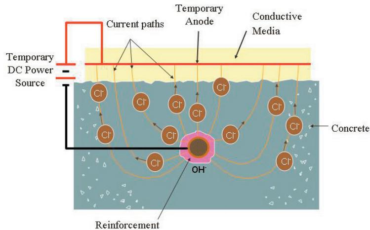
Figure 5: Electrochemical Chloride Extraction (ECE) System
