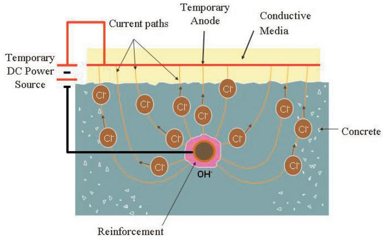
Figure 5: Electrochemical Chloride Extraction (ECE) System
