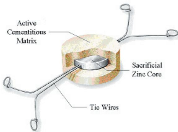
Figure 3: Cut-Away Diagram of Embedded Galvanic Anode
