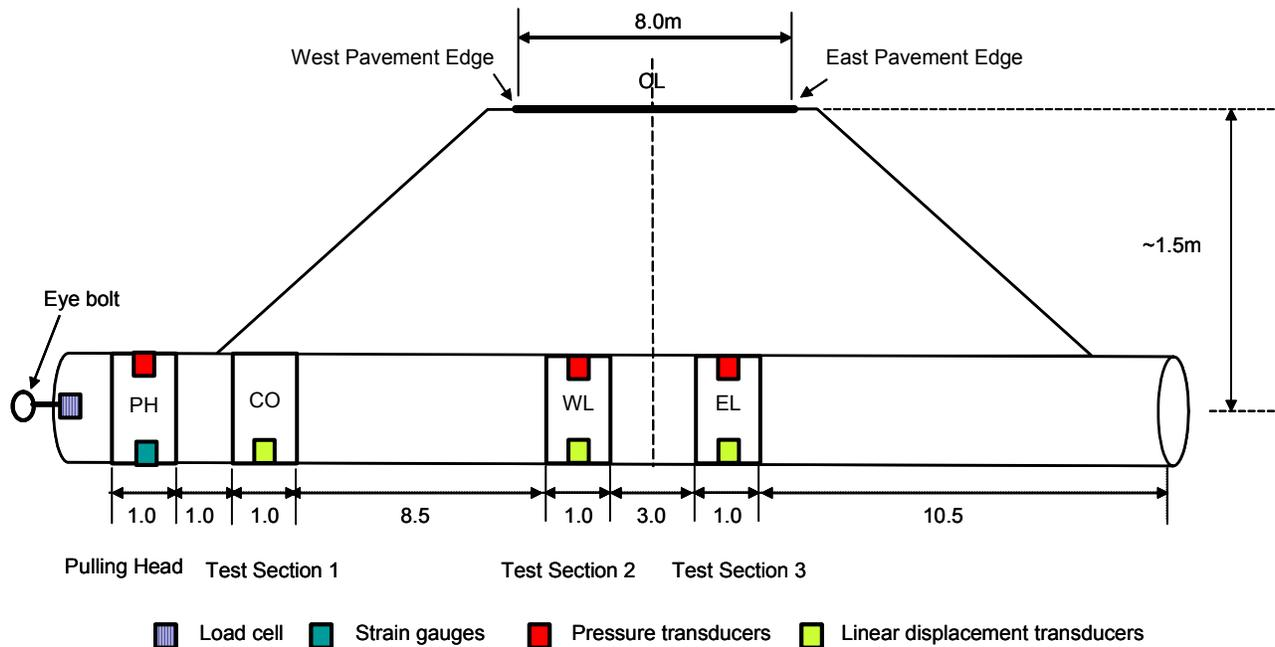
Figure 3: Layout of the 20 sensors placed inside the HDD installed pipe.
