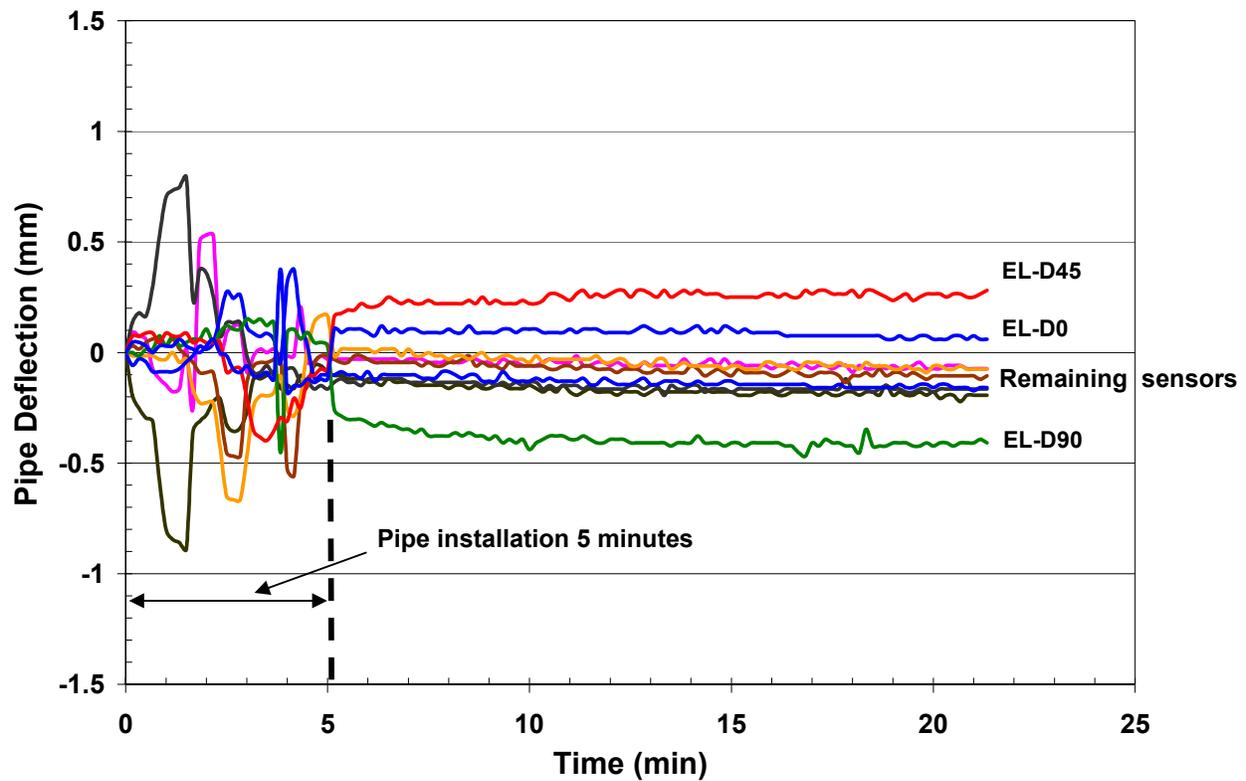
Figure 6: Horizontal directional drilled HDPE installation ring deflections.
