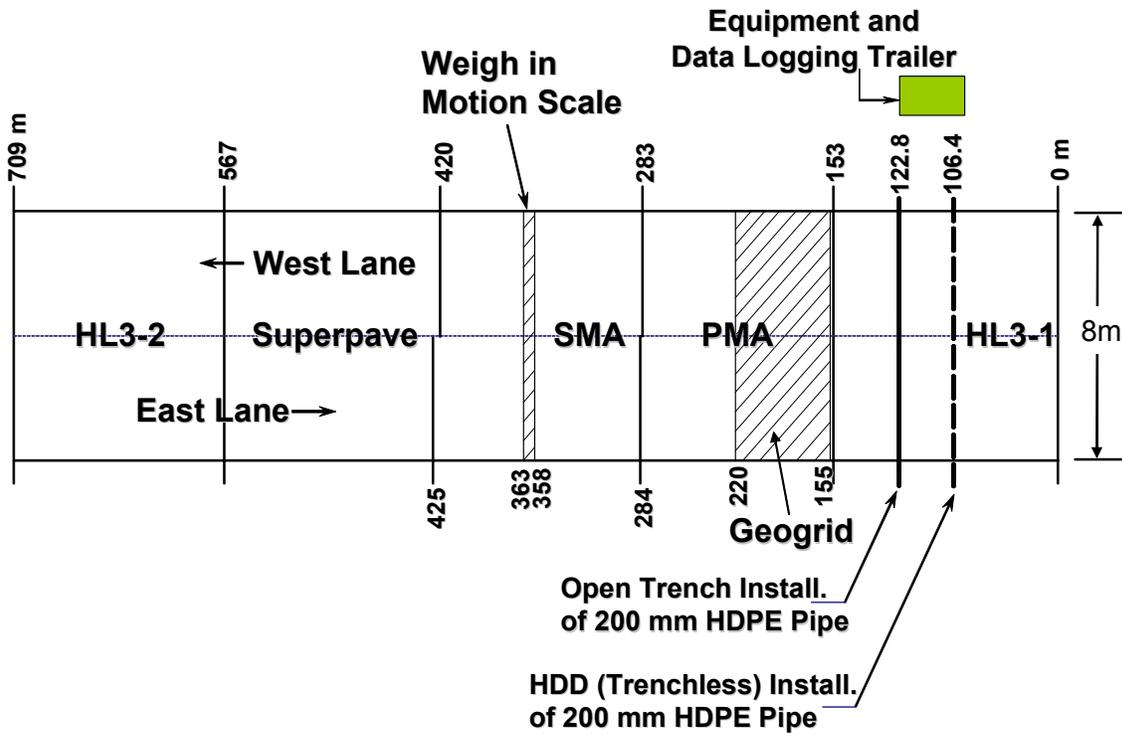
Figure 2: Test track layout.
