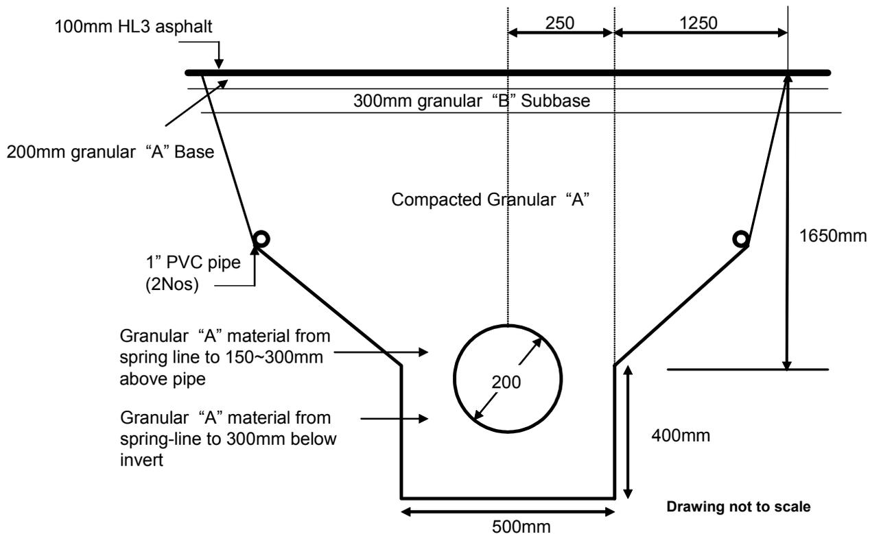
Figure 4: Open cut trench construction geometry and pipe location.
