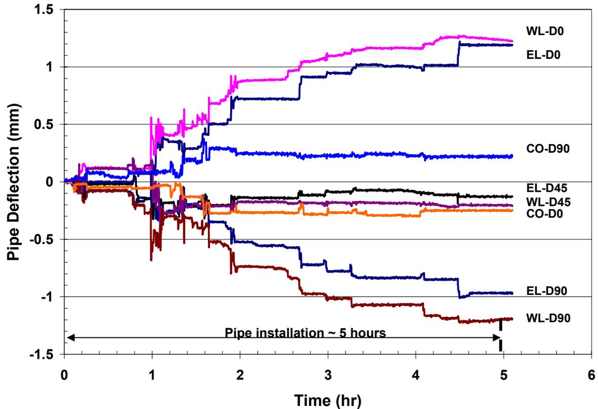
Figure 7: Open cut HDPE installation ring deflections.
