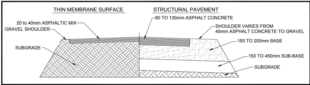
**Figure 2 - Comparison of a Typical Thin Membrane Surfaced Cross-Section with a Structural Pavement**
