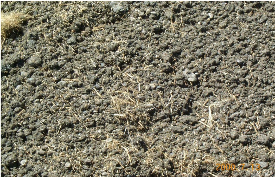
**Figure 9 – Geocomposite of Flax Straw and In Situ Material**
