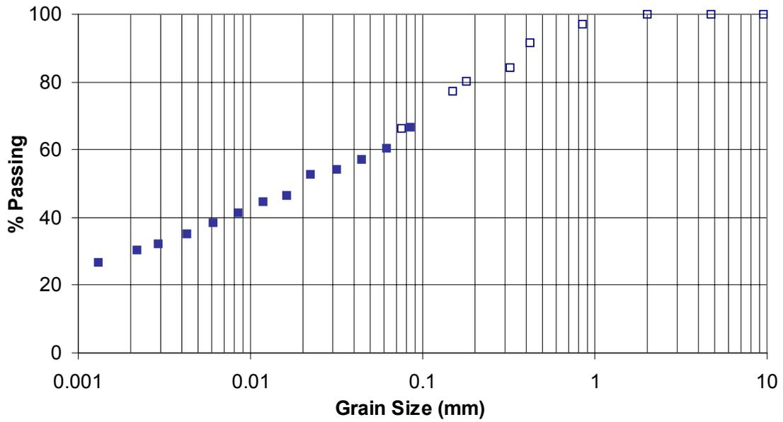
**Figure 5 – Grain Size Distribution of Subgrade Material on Highway 19**
