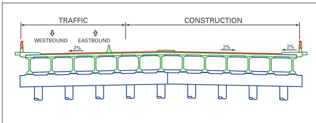
Figure 6 – Stage Three – Construction of Remaining Portion of Proposed Bridge
