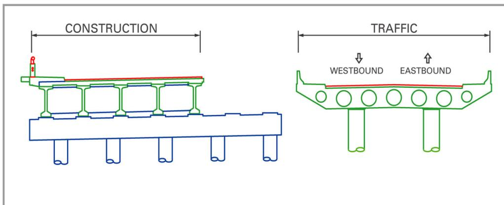
Figure 4 - Stage One - Construction of North Portion of Proposed Bridge
