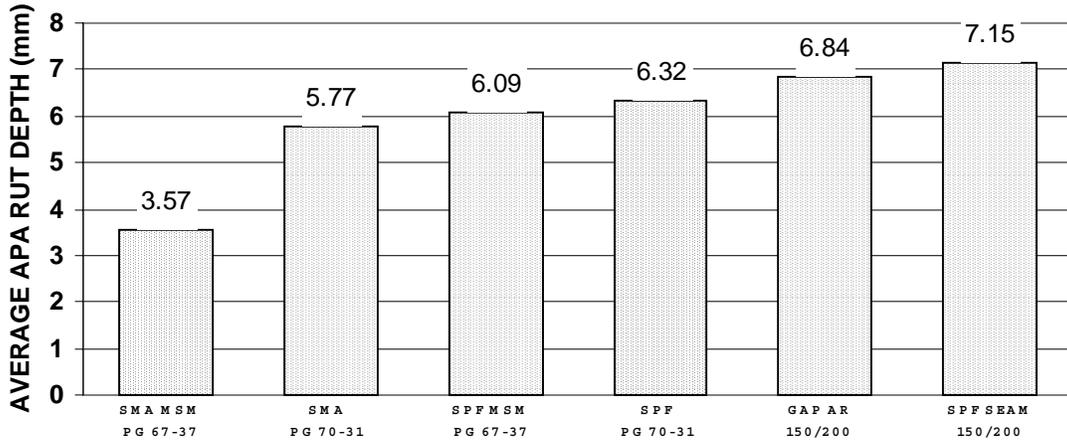
Although this comparison is generally consistent with “expected performance”, some inconsistencies are evident. For example, the rut depth of the two Superpave mixes with similar high temperature binder characteristics is similar, but the rutting depth of the two SMA mixes is not similar.
