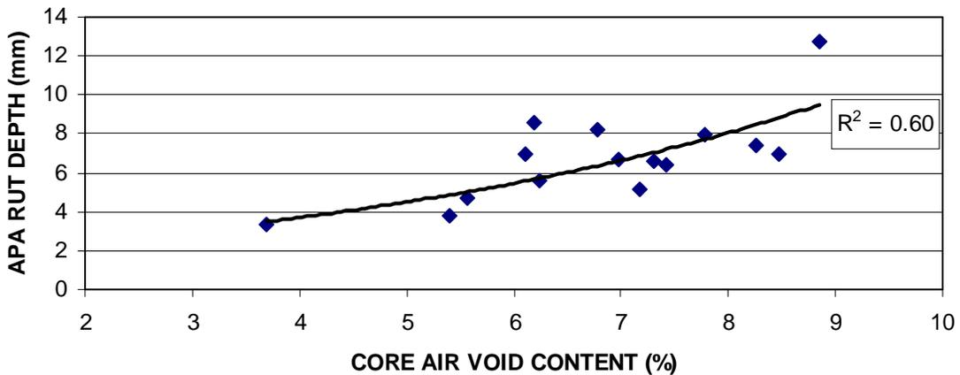
Although only a fair correlation exists ( $R^2=0.60$ ), there appears to be a clear trend that as air void content increases the APA rut depth increases. Based on this limited data, core samples with air void contents greater than 7% when tested using the APA may not provide a good indication of rutting susceptibility. This is most likely the case when this air void level is not typical of the installation.
