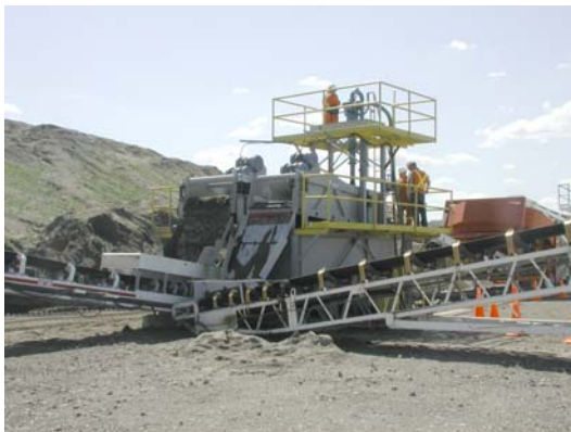
Cyclone & dewatering screens
