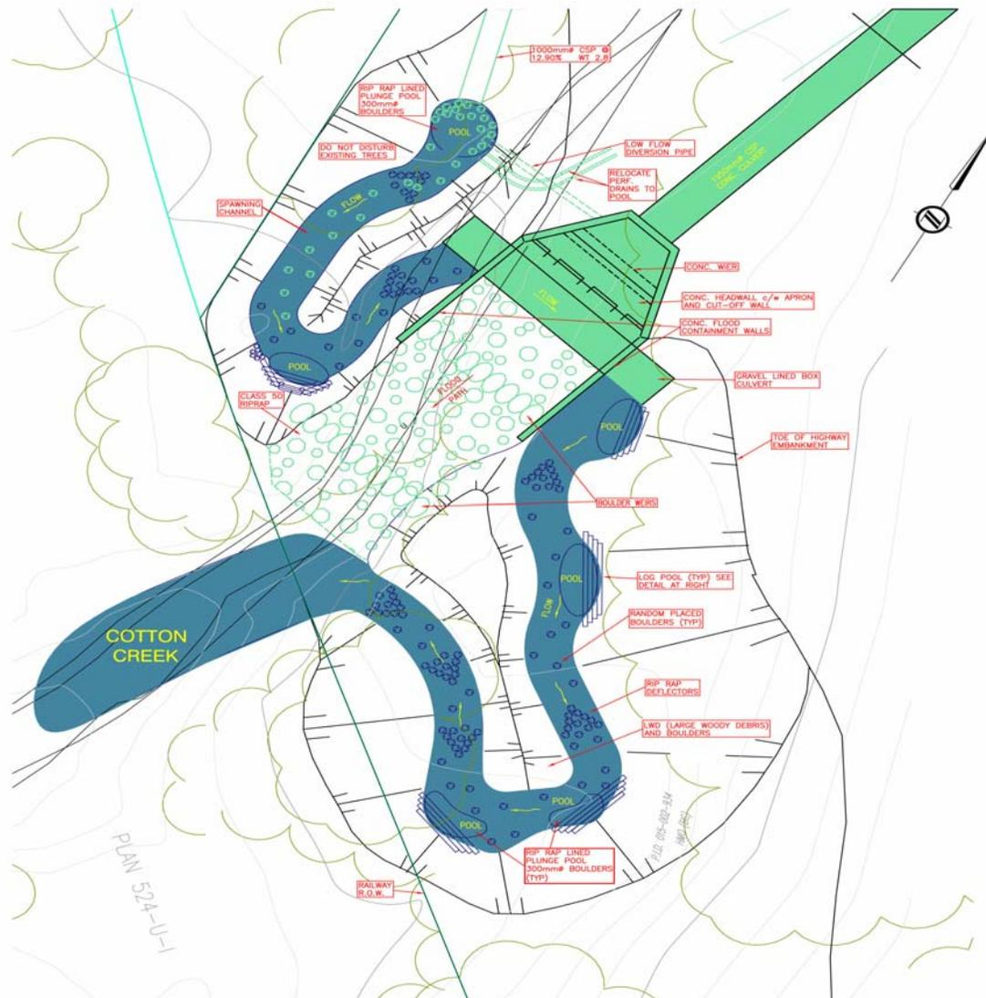
**FIGURE 4 – ENVIRONMENTAL ENAHNCEMENT DETAILS**
