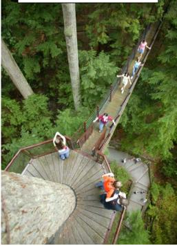
To support the viewing platforms at each tree we designed unique friction collars. Tension bolts on these collars are precisely torqued to generate friction on the tree trunk of 20 pounds per square inch – roughly the pressure the average person can exert by pushing down firmly on a table top with their thumb. Thanks to this design, the platforms can easily support visitors standing shoulder to shoulder on every platform and every bridge, without causing any damage
