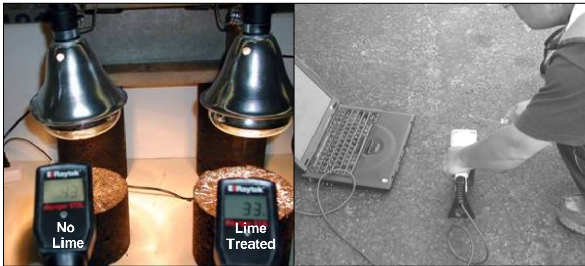
Photograph 9. Laboratory Surface Temperature Testing of Asphalt Concrete Specimens (Left) and Field Testing of Asphalt Concrete Pavement With Impact-Echo Equipment (Right)
