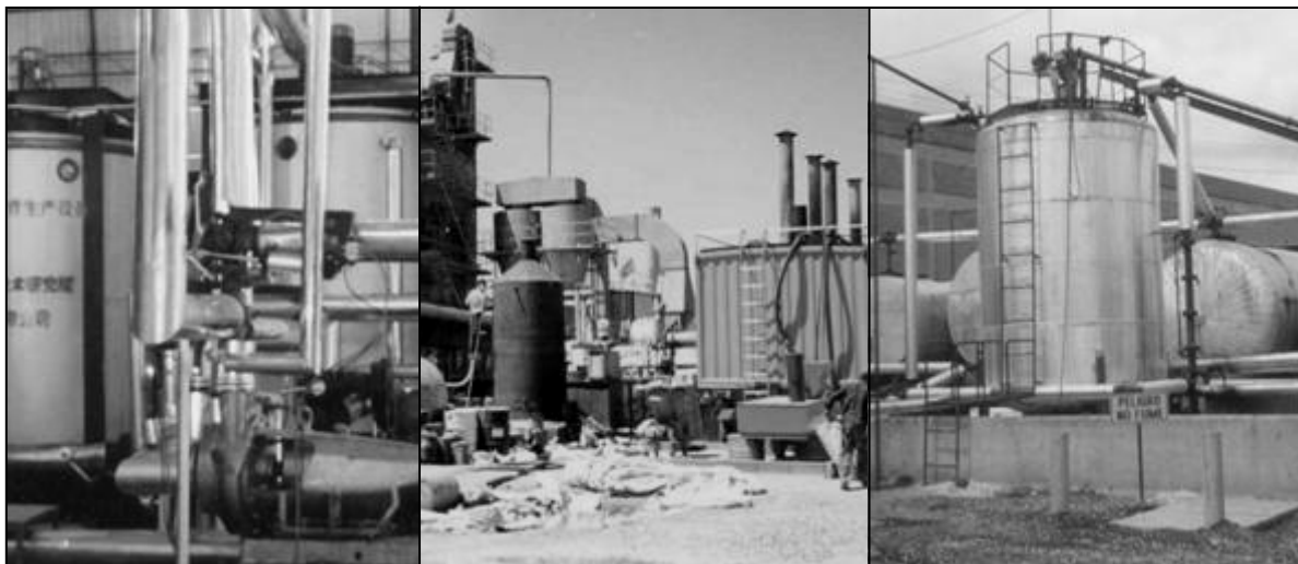
Photograph 4. Typical Polymer Modified Asphalt Cement (Binder) Central and Portable Blending Plants Incorporating Three to Six Percent Styrene Butadiene (SBS) Linear Block Copolymers
