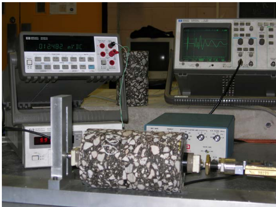
Figure 6: Ultrasonic pulse velocity (UPV) test
