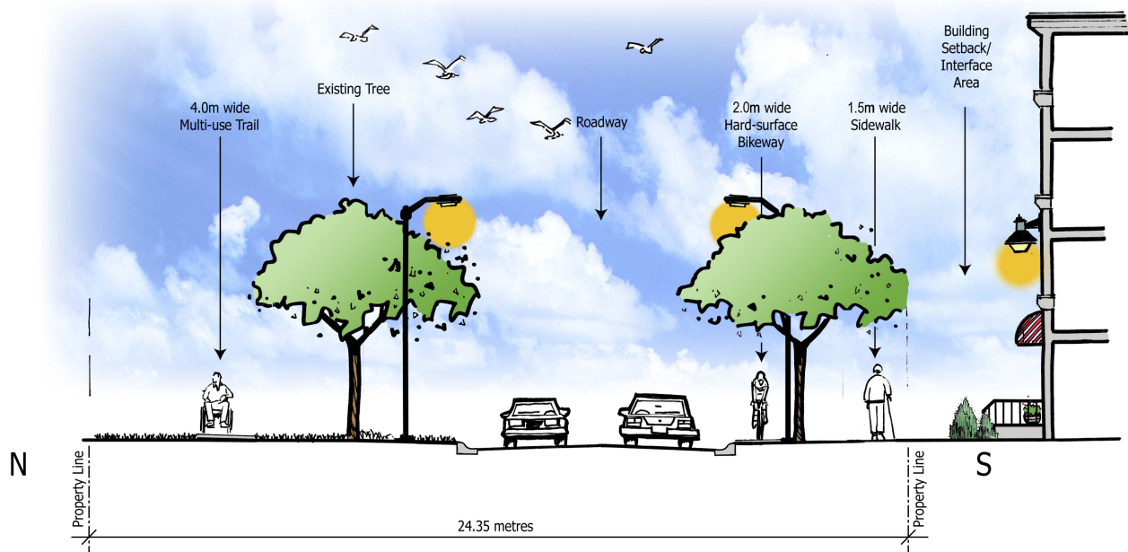
Figure 4a – Proposed Roadway Cross-Section 116 Street to 119 Street
