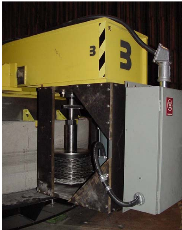
Figure 10 Grinding Unit Attached to TPTA with One Wheel Track of Blades Attached
