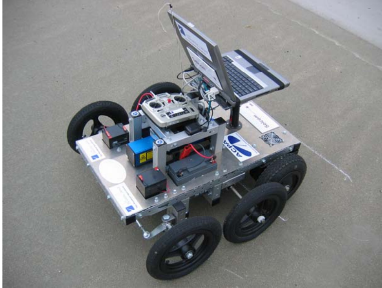
Figure 15 Photo of Robotec 3D Texture Measurement System 10
