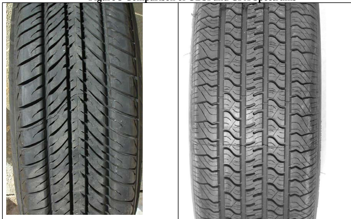
Figure 6 Comparison of Goodyear Aqua Tread (left) and ASTM SRTT Tires (Right)
