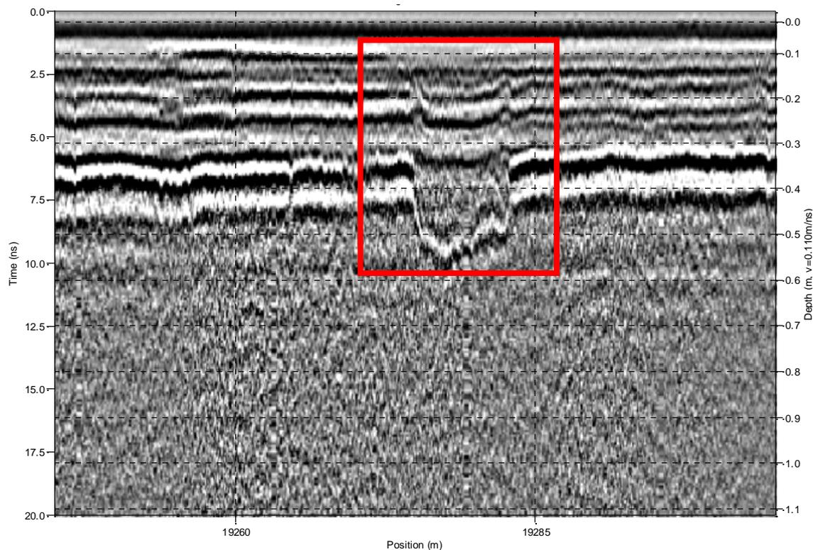
Figure 7 – Example of full depth asphalt repair of a failed concrete slab
