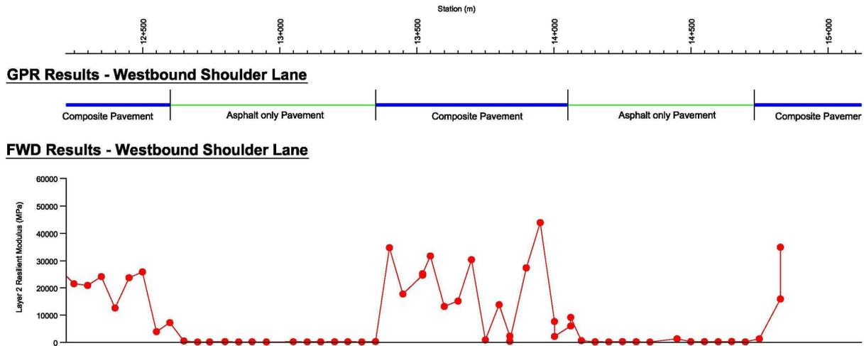
Figure 9 – Comparison of GPR and FWD results for the QEW Westbound Shoulder Lane
