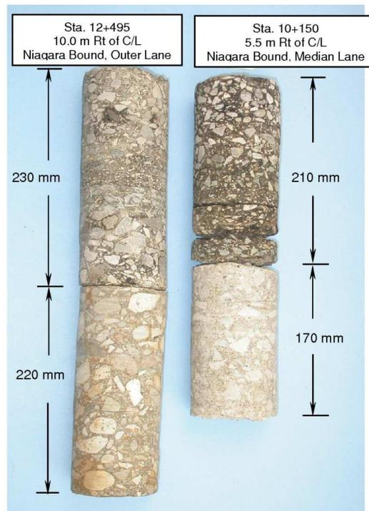
Figure 4 – Typical Core samples from the QEW
