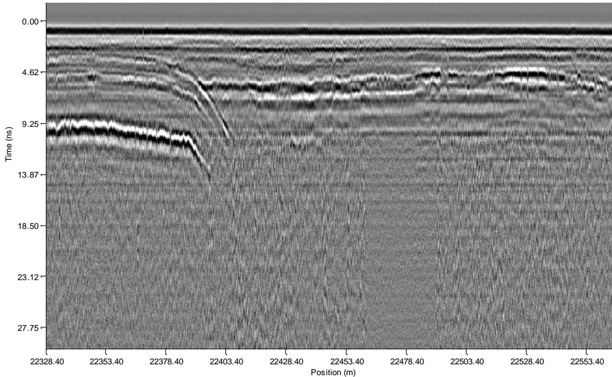
**Figure 5 – Example of Raw Collected QEW GPR Data - Uninterpreted**
