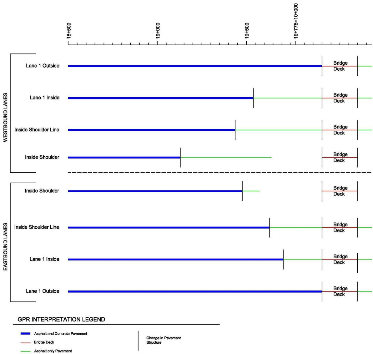
**Figure 8 – Plan summary of GPR results for a portion of the QEW identifying an historical change in highway alignment (Blue is for composite pavements and Green is for flexible pavements)**
