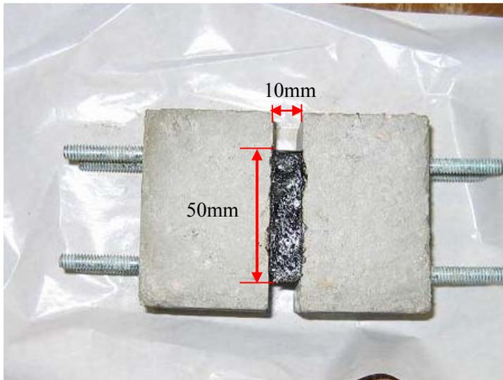
**FIGURE 1: Sealant Specimen for Cyclic Tension and Compression Test**
