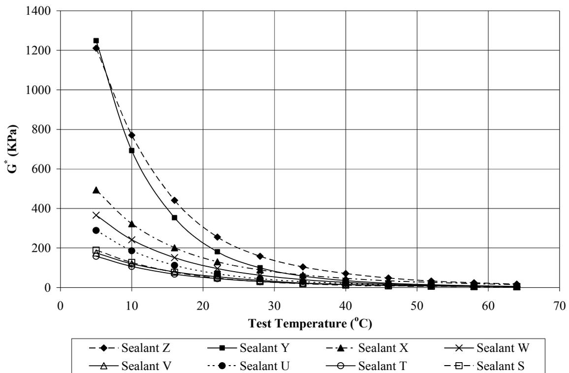
**FIGURE 4: Complex Shear Modulus ( $G^*$ )-Temperature Curve**
