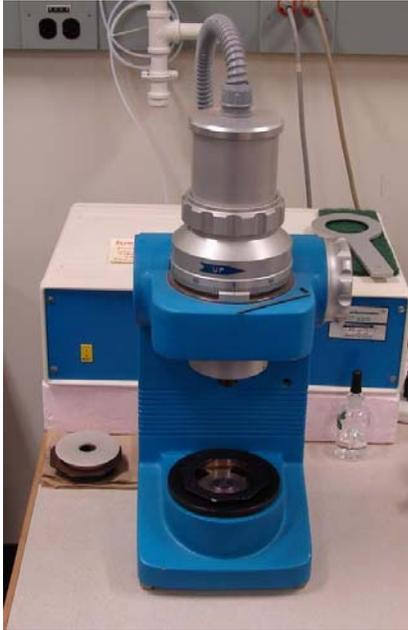
**FIGURE 2: DSR Testing Equipment**
