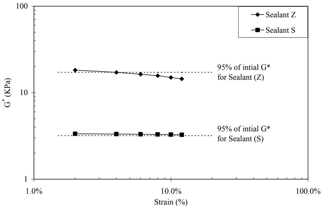
**FIGURE 3: Linearity Check for Sealants (Z) and (S) at +64°C**
