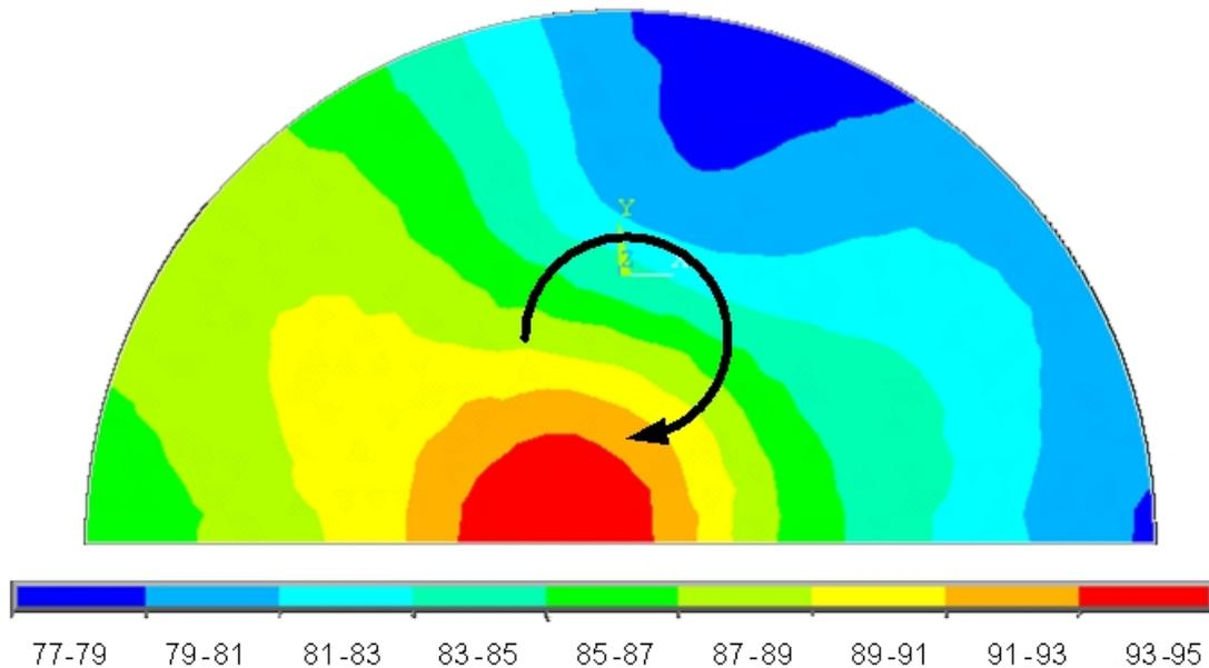
**Figure 7** Sound Intensity mapping around the tire on the ARC pavement at the speed of 80 km/hr and 350 Hz
