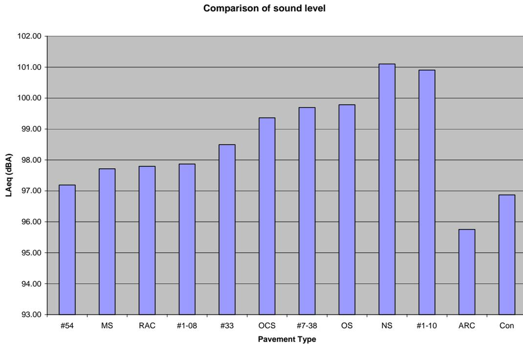
**Figure 5** The comparison of the emission noise level between various surfaces
