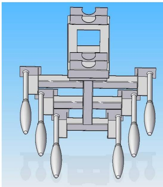
**Figure 2** the drawing of microphones support frame
