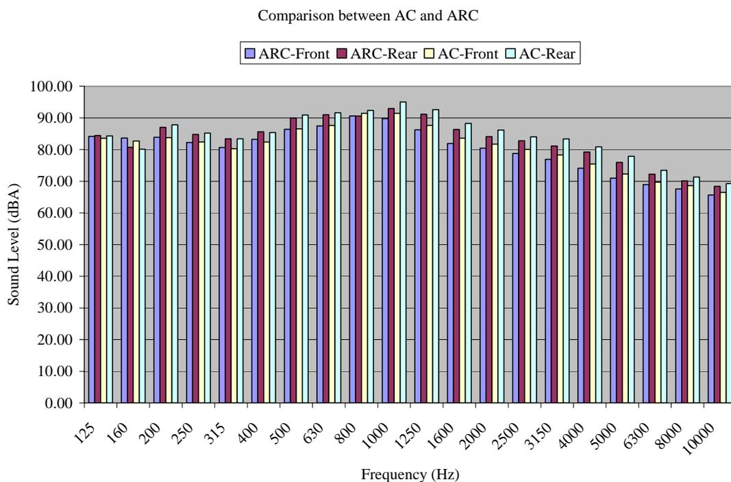
**Figure 4** The comparison between sound level on ARC and AC pavement both at front and rear microphones
