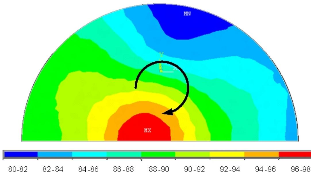
**Figure 6** Sound Intensity mapping around the tire on the AC pavement at the speed of 80 km/hr and 350 Hz
