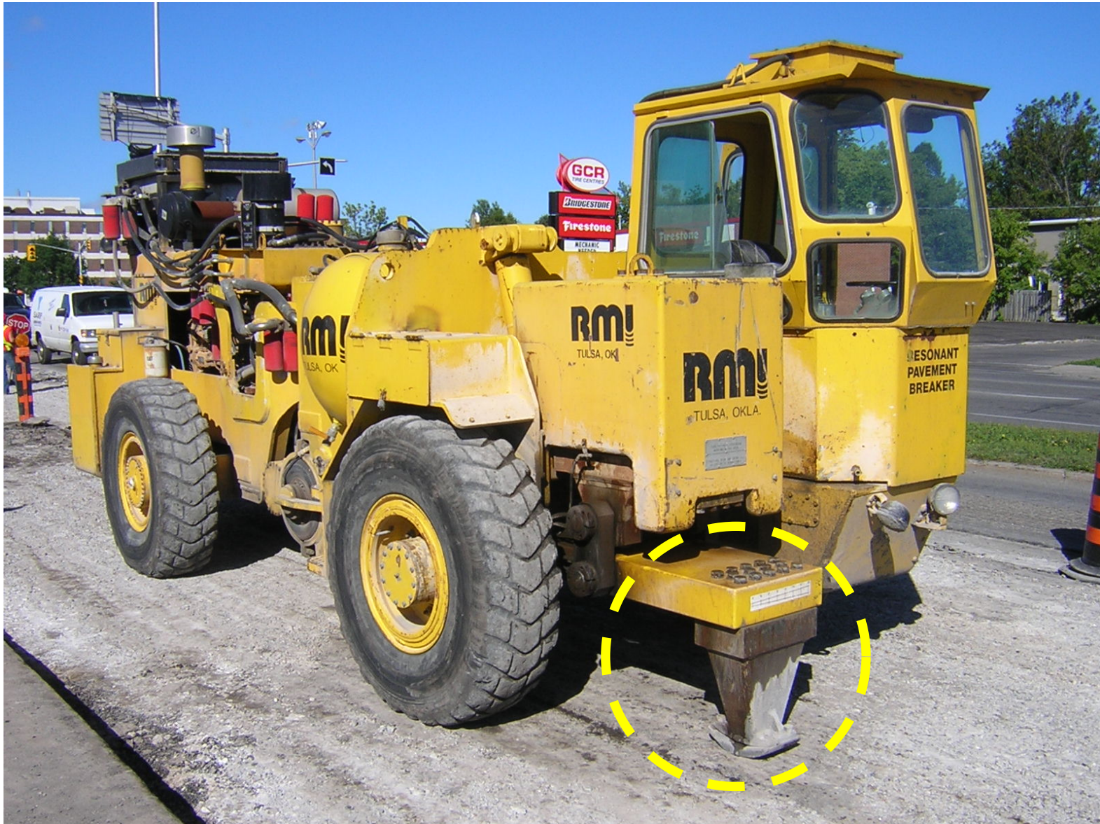
Figure 6: Rubblizer (Dashed Circle highlights single Resonant Breaker Head)
