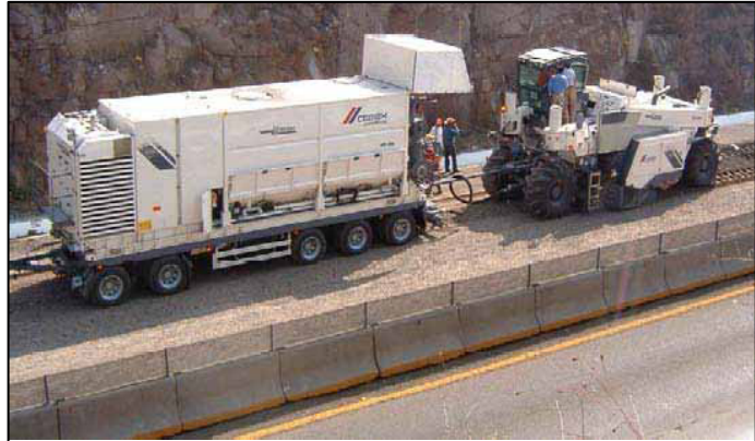
Figure 2.3-1 Wirtgen WM 1000 slurry mixer
