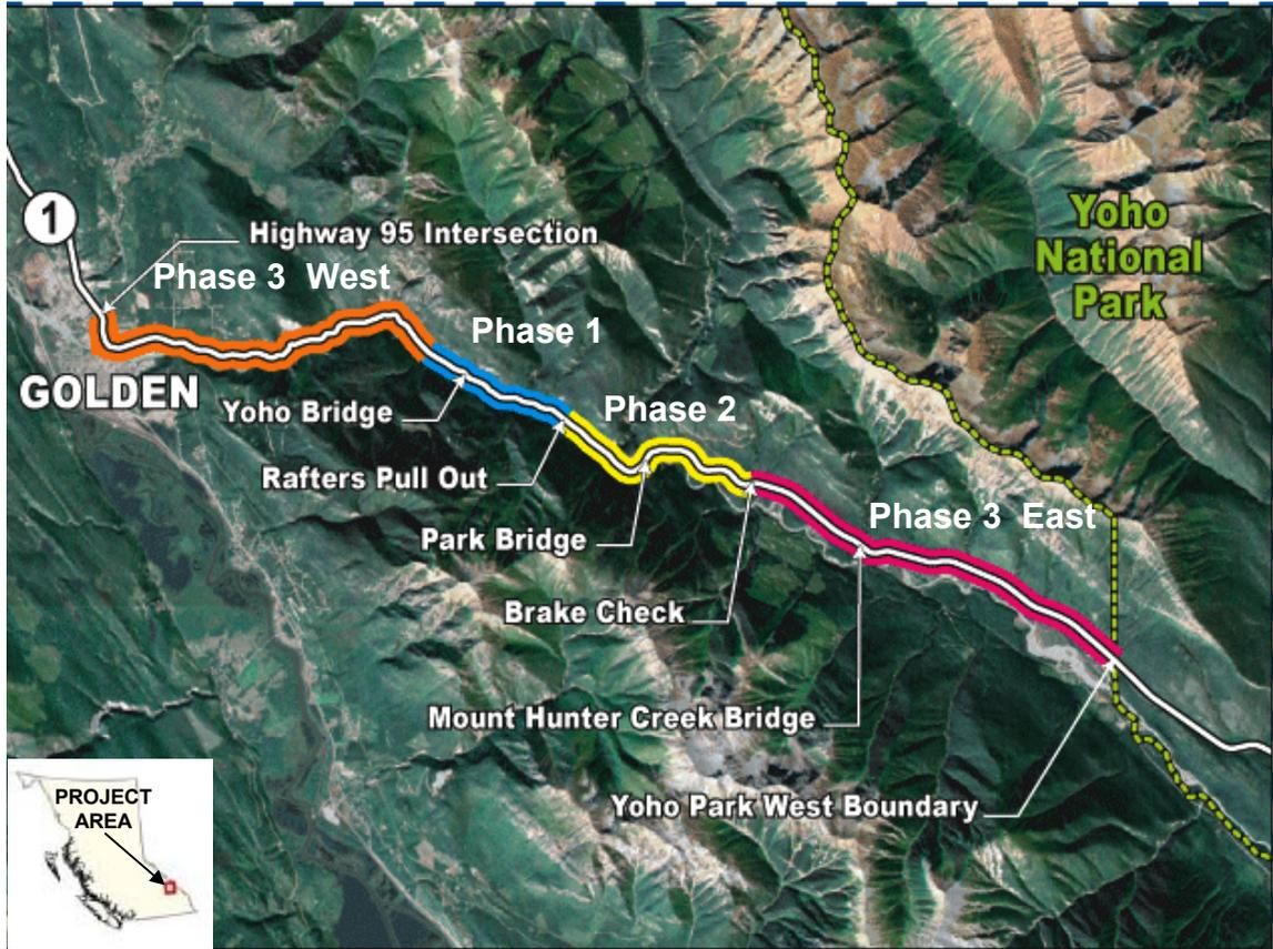
**Figure 1.** Kicking Horse Canyon Project area showing the various construction phases.
