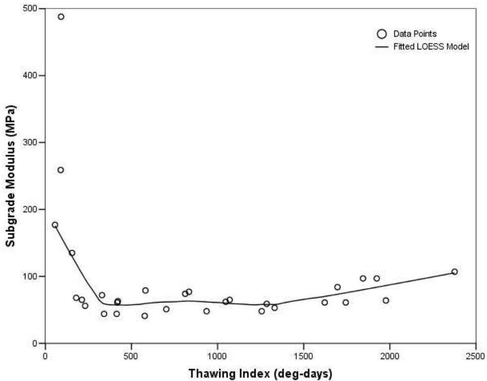
Figure 2 – LTPP Subgrade Modulus vs. Thawing Index
