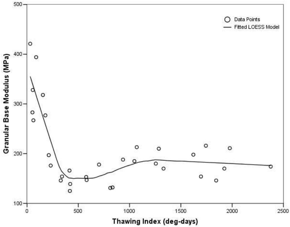
Figure 1 – LTPP Granular Base Modulus vs. Thawing Index
