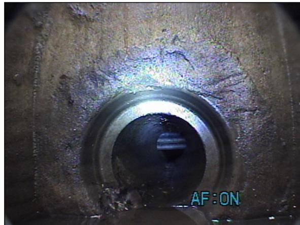
**Figure 6 - Zoom Camera photo showing conduits directionally drilled through Storm Sewer**
