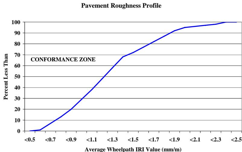
In these situations, the primary criteria require that any 50 m length of pavement where the International Roughness Index (IRI) exceeds 2.5 mm/m be repaired to improve the ride quality. The second criteria requires that the distribution of roughness values for the total population of 50 m sections fall into the conformance zone as indicated above.
