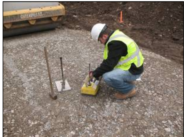
Figure 15a & 15b – Compaction Testing Foundation Improvement – Stage Two
