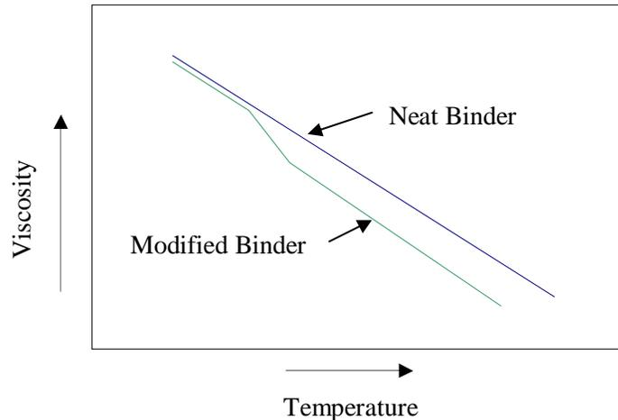
Figure 3 – Modification of binder temperature/viscosity relationship
