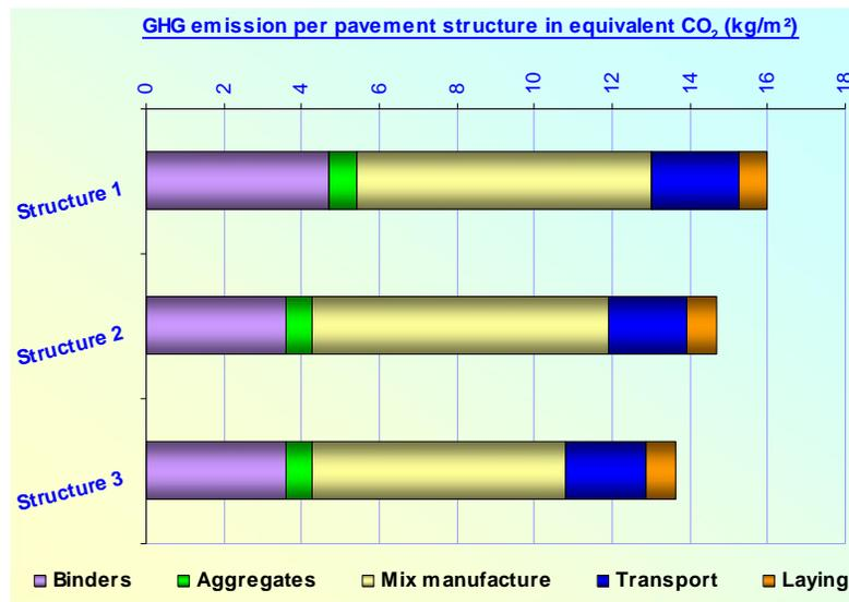
Figure 2 – Output of “EcologicieL” comparing greenhouse gas emission in CO<sub>2eq</sub> (kg/m<sup>2</sup>) of traditional virgin HMA (Structure 1), recycled HMA (Structure 2) and recycled WMA (Structure 3)
