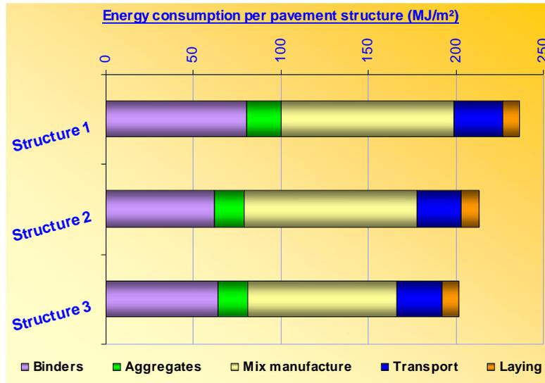
Figure 1 – Output of “EcologicieL” comparing energy consumption (MJ/m<sup>2</sup>) of traditional virgin HMA (Structure 1), recycled HMA (Structure 2) and recycled WMA (Structure 3)
