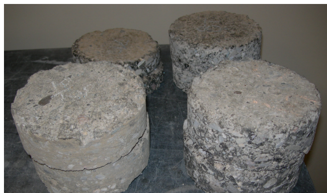
Photograph 7 Cores of granular pavement stabilized with modified foamed asphalt (A) and conventional foamed asphalt (B).
