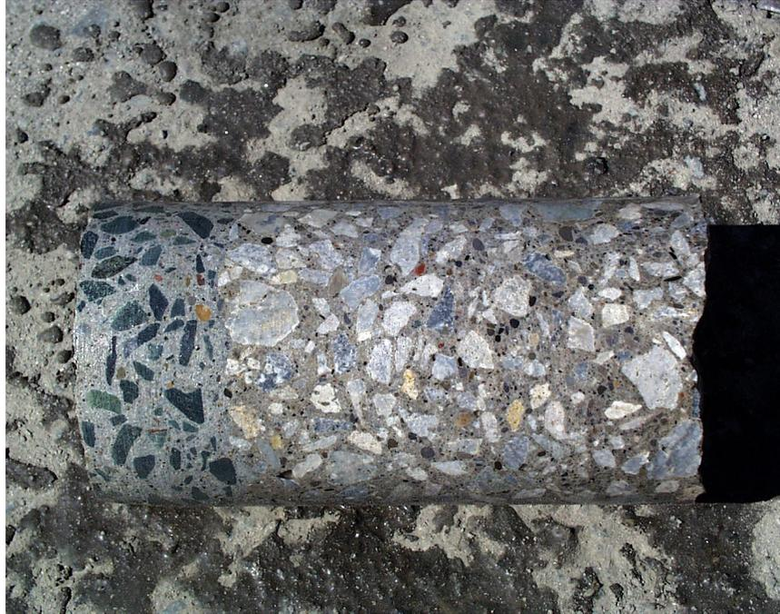
**Figure 10 Core taken from deck with latex modified overlay**
