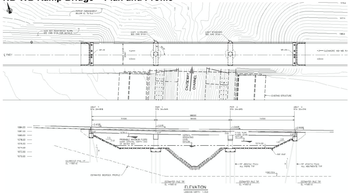
The two bridges are essentially the same in profile with the difference being shortening the west span to avoid conflicting with the West Pumphouse as illustrated below.
