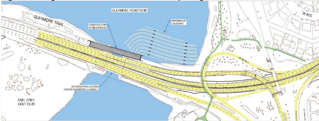
Figure 7 – Stage 2 – Remove and Construct EB Half of Causeway Bridge
