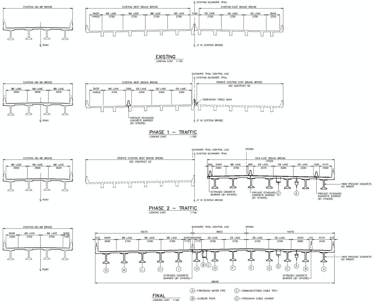
Stage 2 (Fig. 7) which removed the existing and enabled construction a new Eastbound Causeway Bridge occurred from November 2006 through October 2007. During this time construction activities were by and large confined to a work zone on the south side of the remaining westbound half of the existing bridge. The number of lanes available
