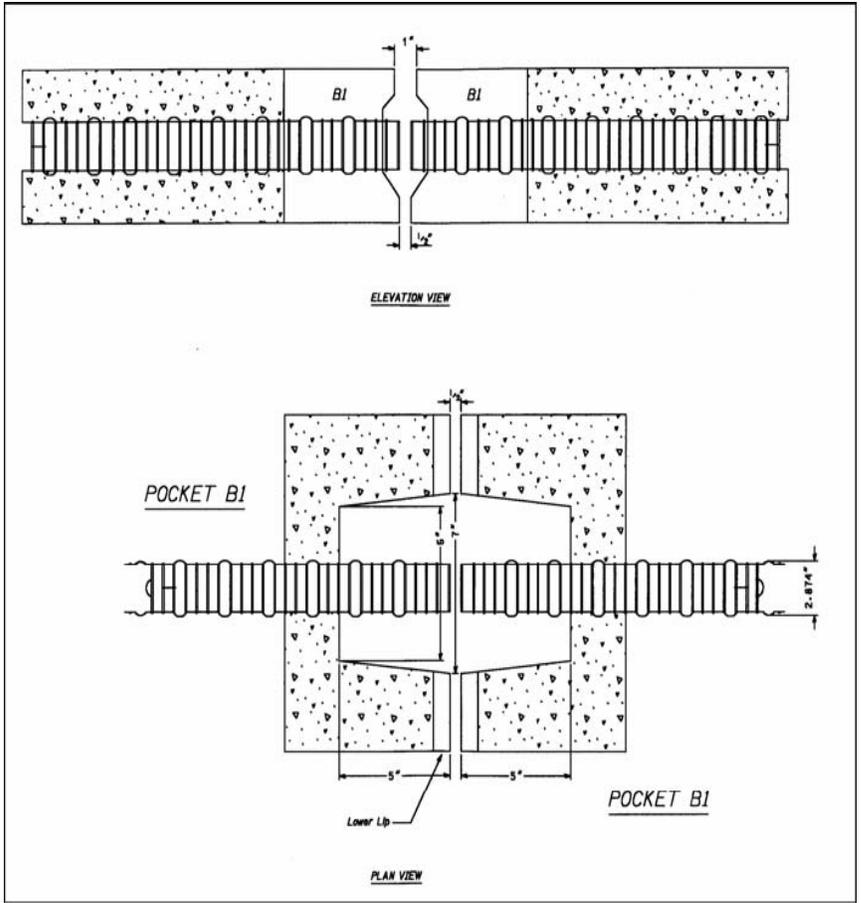
Figure 7 – Typical layout of sheath ducts across a transverse joint
