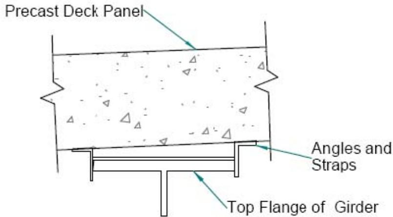
**Figure 9 – Levelling and haunch forming system on steel girders**
