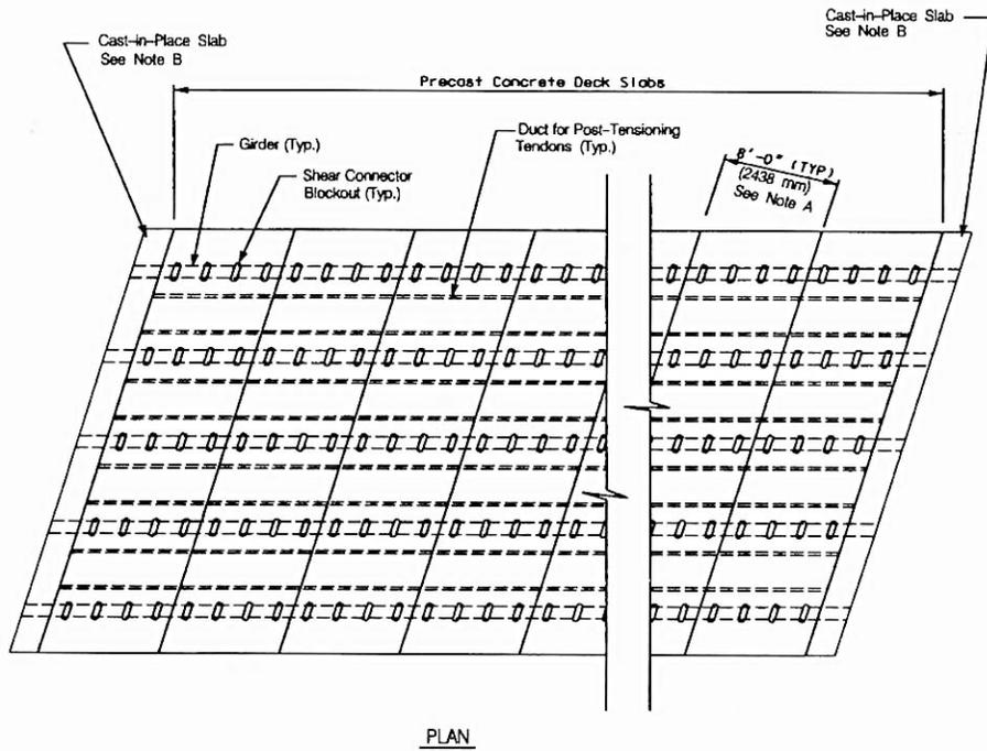
**Figure 1 – Plan view of typical deck panel layout**
