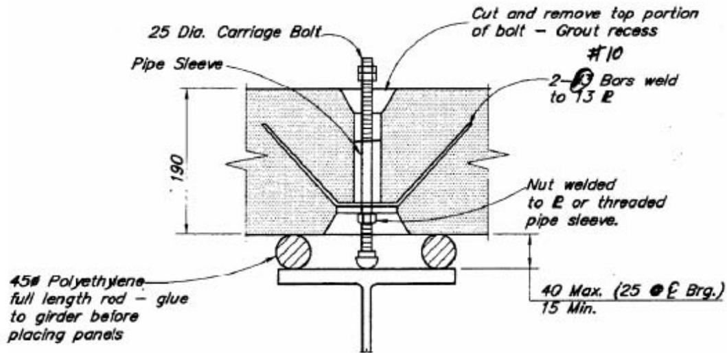
Figure 5 – Leveling bolt detail
