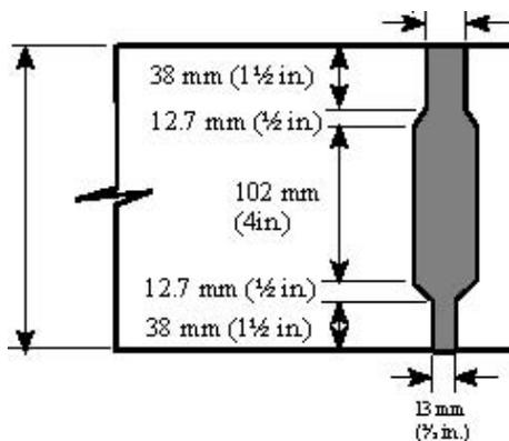
**Figure 11 – Typical female-to-female transverse joint**
