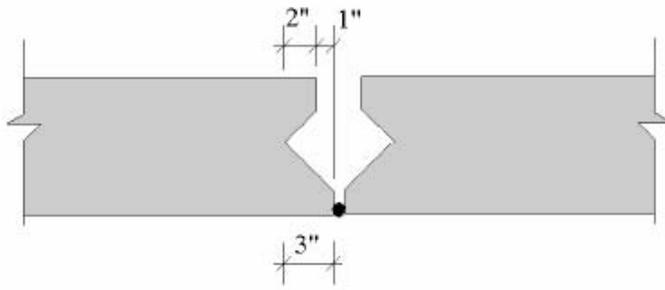
**Figure 12 – V-shaped shear key used in Nebraska**
