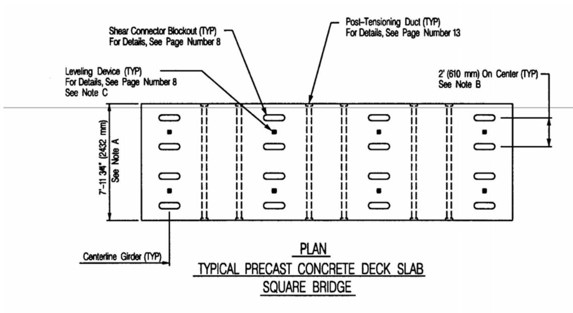
**Figure 2 – Typical plan for square panel**
