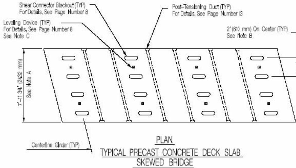
Figure 3 – Typical plan for skewed panel
