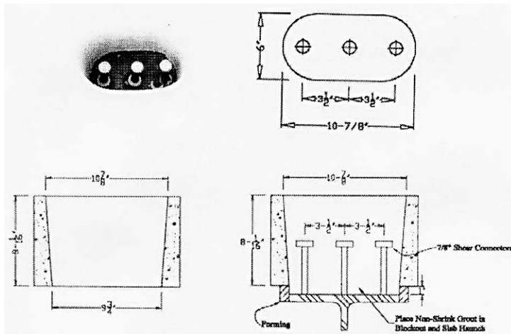
Figure 4 – Shear stud and pocket detail
