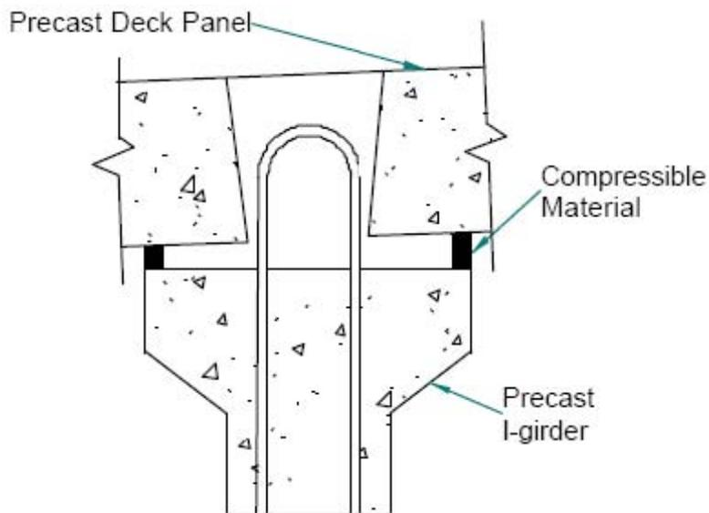
**Figure 10 - Levelling and haunch forming system on precast concrete girders**
