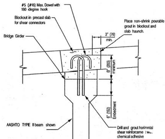
Figure 8 – Section view of shear connector for precast concrete girders
