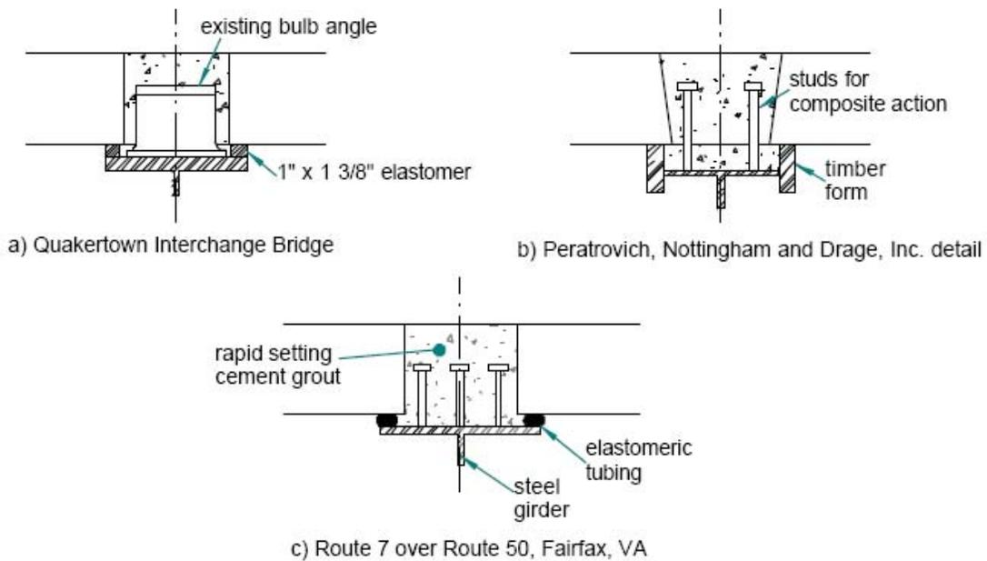
Figure 6 – Haunch forming details used on various bridges
