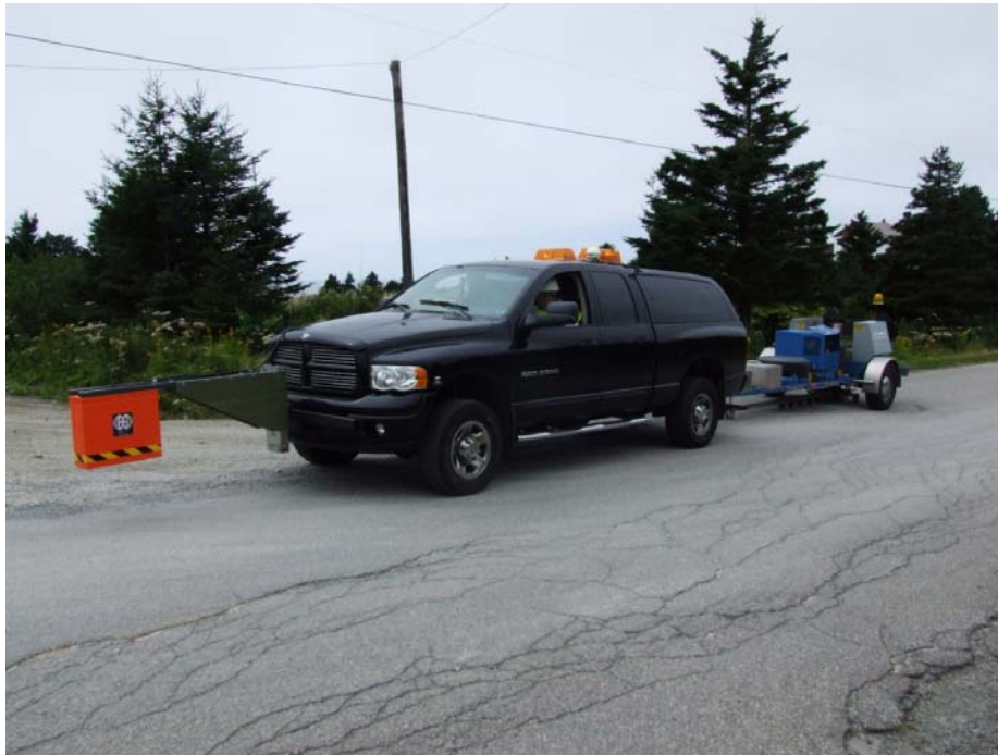
Figure 1 - Simultaneous GPR and FWD data collection on the pre-rehabilitation pavement surface.
