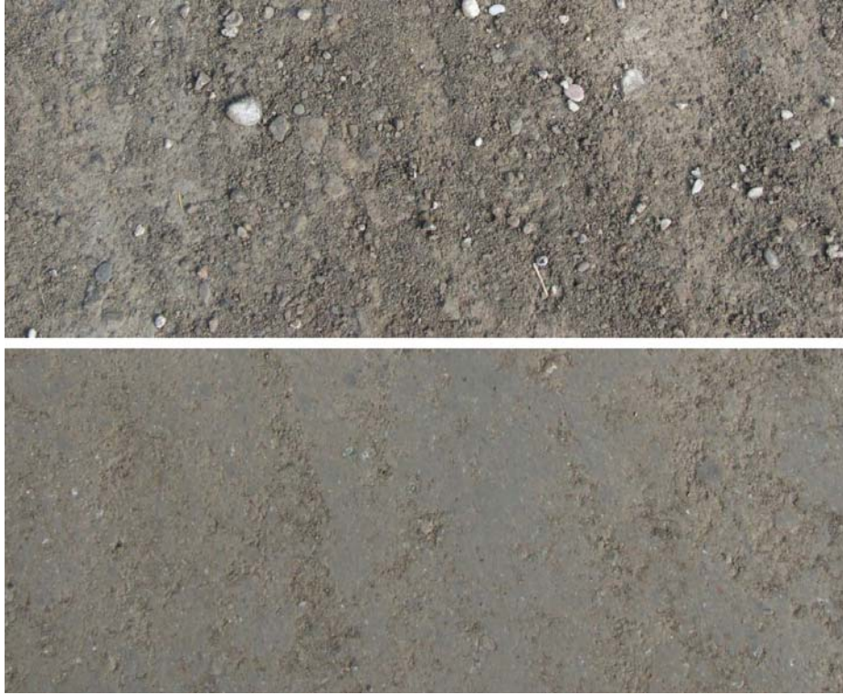
Figure 9 - Comparison between pre-microcracked (top) and post-microcracked (bottom) PC-FDR.
