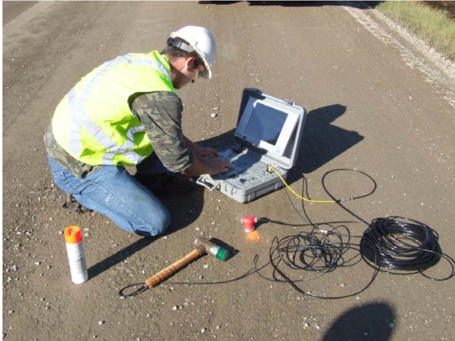
Figure 7 - Slab IR test system used to measure PC-FDR pavement stiffness.
