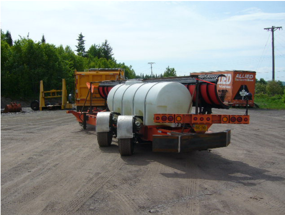
Figure 5 – Modifications including cycle fenders, chamfered bumper
