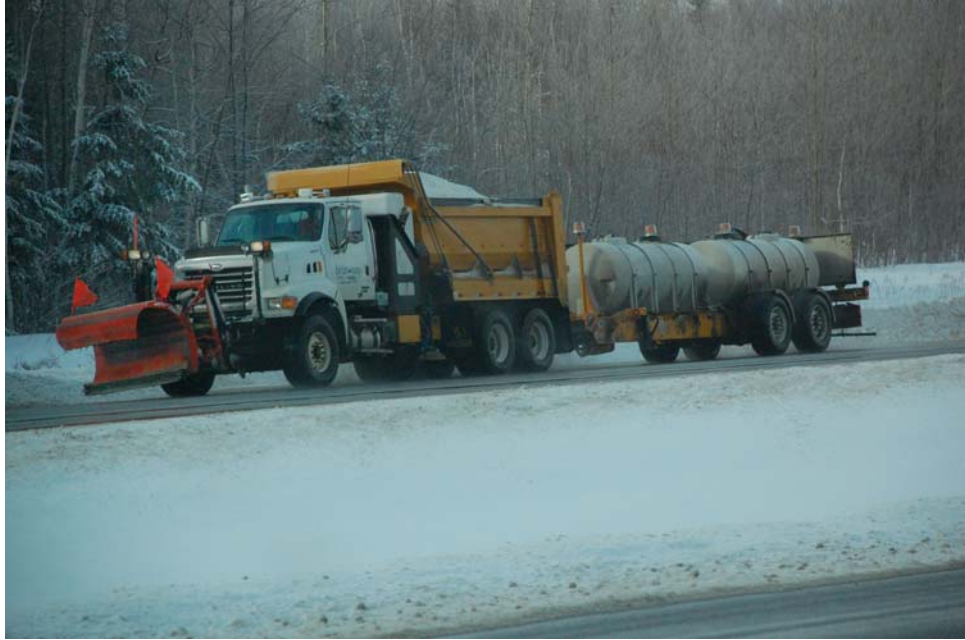
Figure 4 – Anti-Icing with Tow Plow
