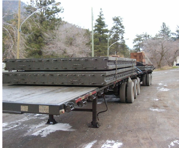
Photo 5: Concrete Wall Panels
